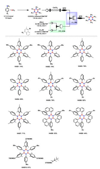
Fig. 3 HABs synthetized under continuous flow process. Reaction conditions: Ar–Br (0.18 M in 2-MeTHF), n-BuLi (0.5 M in hexane/2-MeTHF), and TCB solution (0.05 M in toluene/heptane/2-MeTHF) produced from aniline derivatives (1.0 equiv.); BCl $_3$  (1.2 equiv.) were introduced to the flow system fabricated by PEEK Tee (ID: 0.5 mm) and PTFE tube ( $\emptyset$ i.d.: 1 mm) using high-pressure syringe pump, isolated yield over two steps.
