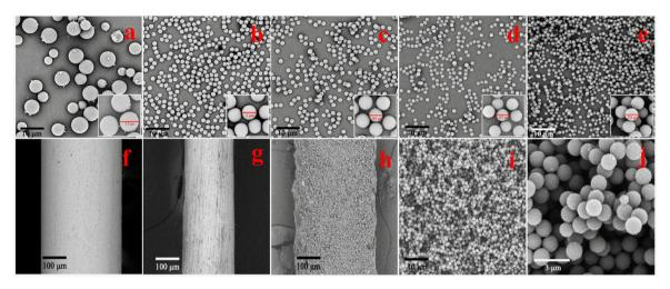
Fig. 2 SEM images of the MFRs (a-e) with a PVP quality of 0, 0.10, 0.30, 0.50, and 0.70 g, respectively. SEM images of the fiber (f) before and (g) after corroding by using agua regia; SEM images of the MFR-based SPME fiber at different magnifications: (h) ×500; (i) ×5000; (j) ×25000.
