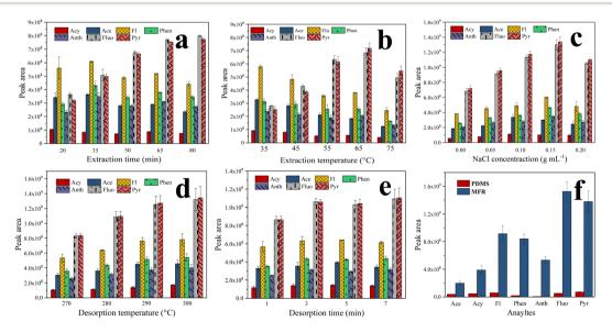
Fig. 4 Effects of SPME conditions on the extraction efficiencies: (a) extraction time; (b) extraction temperature; (c) NaCl concentration; (d) desorption temperature; (e) desorption time; and (f) comparison of the enrichment efficiencies of PDMS and the MFR.
