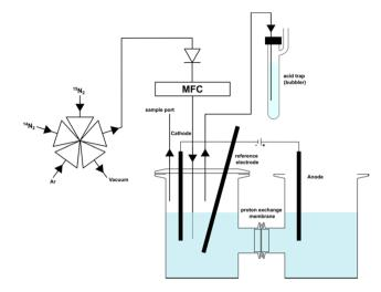
Fig. 1 Schematic representation of the setup used for studying the NRR under  $^{14}N_2$  or  $^{15}N_2$  atmospheres. NRR experiments were conducted in an H-cell configuration. Feed gases ( $^{14}N_2$  and  $^{15}N_2$ ) were continuously bubbled into the cathode compartment at a predefined flow rate of 20 mL min $^{-1}$ . An acid trap was employed at the exit to completely isolate the cathode compartment from the surrounding atmosphere and to trap any gaseous ammonia.
