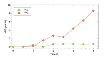
Fig. 2 Cumulative ammonium production ( $^{15}NH_4^+$  or  $^{14}NH_4^+$ ) in a four hour NRR experiment with a Bismuth cathode.
