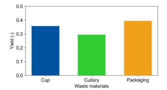
Fig. 4 Yield of lactic acid determined with HPLC for the depolymerisation of real waste materials. Conditions: Pt cathode, Pt anode, 40 mA cm $^{-2}$ , 150 C, dioxane/water (vol. 9:1), 0.25 M LiClO<sub>4</sub>, 60 °C, 5 mg mL $^{-1}$  PLA.
