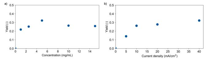
Fig. 2 Yield of lactic acid determined with HPLC for (a) different concentrations (40 mA cm $^{-2}$ ) and (b) different current densities (5 mg mL $^{-1}$ ). Conditions: Pt cathode, Pt anode, dioxane/water (vol. 9:1), 0.25 M LiClO<sub>4</sub>, 60 °C, PLA (48 300 g mol $^{-1}$ ).
