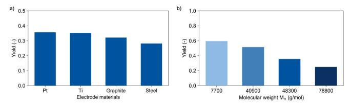
Fig. 3 Yield of lactic acid determined with HPLC for (a) different cathode materials ( $M_n = 48\,300 \text{ g mol}^{-1}$ ) and (b) different molecular weights (Pt cathode). Conditions: Pt anode, 40 mA cm<sup>-2</sup>, 150 C, dioxane/water (vol. 9 : 1), 0.25 M LiClO<sub>4</sub>, 60 °C, 5 mg mL<sup>-1</sup> PLA.
