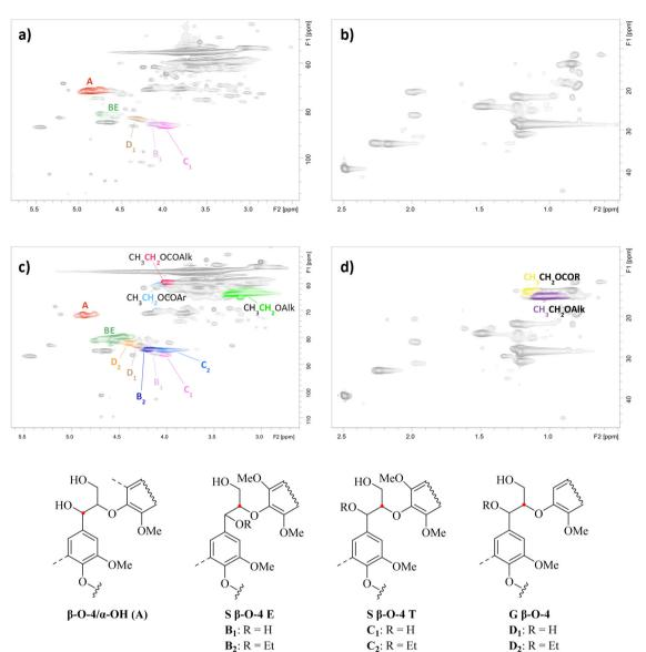
Fig. 3 2D HSQC spectra of ethanol extracted lignin (EEL; a and b) and reactive extracted lignin (REL; c and d). Reaction conditions to produce REL: t = 4 h, [EtOH] = 99%, [H<sub>2</sub>SO<sub>4</sub>] = 0.15 M, T = reflux.
