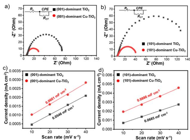
**Fig. 5** Nyquist plots of (a) the (001)-dominant TiO<sub>2</sub> and (001)-dominant Cu-TiO<sub>2</sub> and (b) the (101)-dominant TiO<sub>2</sub> and (101)-dominant Cu-TiO<sub>2</sub>. The insets are the equivalent electrical circuits. Charging current density plotted against the scan rate at 0.655 V vs. RHE for (c) the (001)-dominant TiO<sub>2</sub> and (001)-dominant Cu-TiO<sub>2</sub>, and (d) the (101)-dominant TiO<sub>2</sub> and (101)-dominant Cu-TiO<sub>2</sub>.
