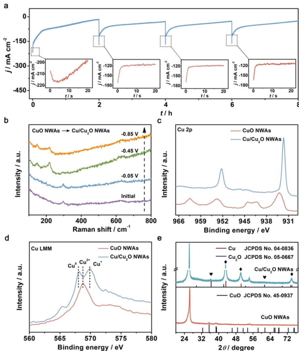
**Fig. 10** (a) The  $i$ - $t$  curves of CuO NWAs during four consecutive cycling NRA processes at  $-0.85$  V. Insets: enlarged details in the dotted box. (b) *In situ* electrochemical Raman spectra of CuO NWAs under given potentials. (c) Cu 2p XPS spectra of CuO NWAs and Cu/Cu<sub>2</sub>O NWAs. (d) Cu LMM AES spectra and (e) XRD patterns of CuO NWAs and Cu/Cu<sub>2</sub>O NWAs. Reprinted with permission from ref. 50. Copyright 2020 Wiley-VCH Verlag GmbH & Co. KGaA, Weinheim.
