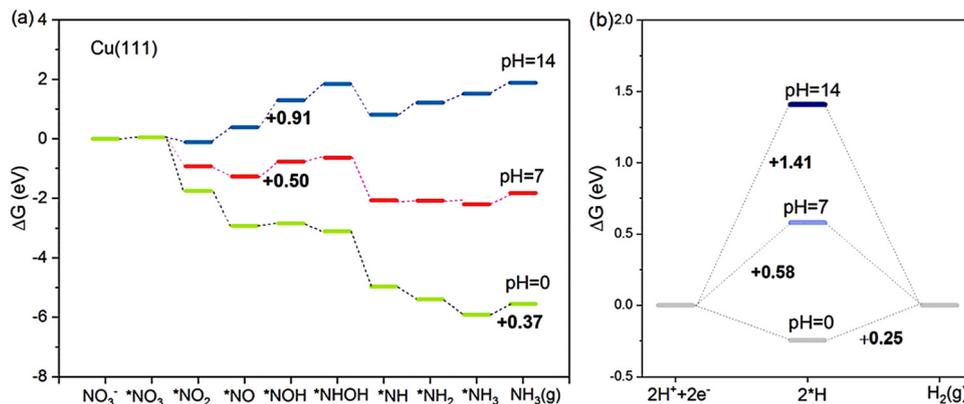
Fig. 4 The competition between (a)  $\text{NO}_3\text{RR}$  and (b) HER on Cu (111) at pH = 0, 7 and 14, studied by Hu *et al.* Reprinted with permission from ref. 33. Copyright 2021, American Chemical Society.
