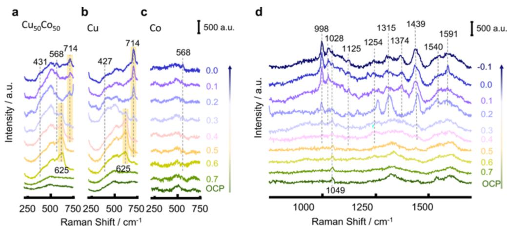
Fig. 16 SHINERS spectra between 230–750 cm<sup>-1</sup> on (a) Cu<sub>50</sub>Co<sub>50</sub>, (b) Cu, and (c) Co. (d) SHINERS spectra between 750–1700 cm<sup>-1</sup> on Cu<sub>50</sub>Co<sub>50</sub> in 100 mM KNO<sub>3</sub> + 10 mM KOH during cathodic polarization from 0.7 to –0.1 V, by Fang *et al.* Reprinted with permission from ref. 92 Copyright 2022 Springer Nature.
