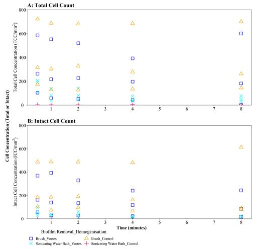
Fig. 4 Cell counts obtained when using different vortexing longevities to homogenise drinking water biofilms removed from sample surfaces by brushing or sonication via a water bath (as indicated in key). Biofilms were 3-months old. Control samples were not vortexed. (A) Total cell counts (TCC) and (B) intact cell counts (ICC) obtained from each BMD section (n = 3) are presented in each panel.
