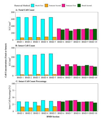
Fig. 3 Comparison of brushing and sonication techniques for removing biofilm from a pipe section (biofilm monitoring device). (A) Total cell counts (TCC) and (B) intact cell counts (ICC) obtained from each BMD section are presented, along with (C) ICC as a proportion of the TCC. Brushing refers to the protocol optimised in this study. Sonication is with glass beads and a water bath.
