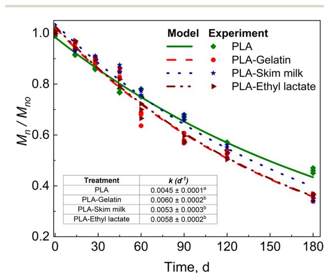
Fig. 2 Normalized  $M_n$  reduction as a function of time for PLA in control compost and compost biostimulated with skim milk, gelatin, and ethyl lactate. The experimental data was fitted using a first-order reaction of the form  $M_n/M_{no} = e^{(-kt)}$ , where  $M_{no}$  is the initial  $M_n$ ,  $k$  is the rate constant, and  $t$  is the time. The inset shows the  $k$ -fitted values; values with different lowercase letters are statistically different ( $\alpha = 0.05$ , Tukey–Kramer test).
