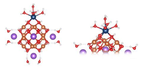
Fig. 2 Ball and stick images of the optimised geometry of the Pu-substituted, Na+-capped, Fe13 Keggin (left); close up of the "square-window" (right). Colour scheme: Pu; blue, Fe, orange; O, red; H, white; Na, purple.
