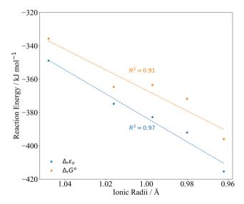
**Fig. 4** PBE0/Def2TZVP/SARC-DKH2 reaction energy  $\Delta_{\rm r}$  according to eqn (2) compared to 8-coordinate An( $\nu$ ) ionic radii. <sup>45</sup>
