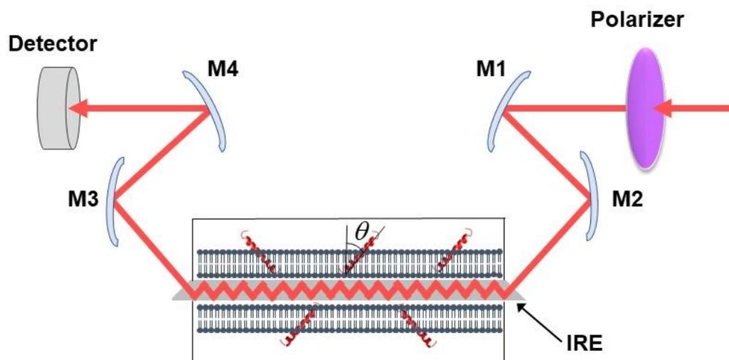
**Figure 1.** Schematic presentation of the ATR-FTIR setting. The infrared light is plane-polarized via a polarizer and directed into the internal reflection element by mirrors M1 and M2. The incident light performs a series of internal reflections, exits the IRE and is directed to the detector by mirrors M3 and M4. The lipid membrane with embedded protein, shown as a single helix, is deposited at both surfaces of the IRE. Reproduced from ref. 94, with permission.
