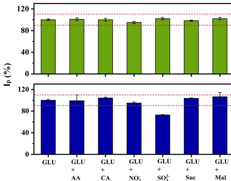
**Fig. 7** Interference study performed by LSV with 1.0 mmol L<sup>-1</sup> glucose (Glu) in the presence of 0.1 mmol L<sup>-1</sup> (green bars) and 0.5 mmol L<sup>-1</sup> (blue bars) of ascorbic acid (AA), citric acid (CA), nitrite (NO<sub>2</sub><sup>-</sup>), sulphite (SO<sub>3</sub><sup>2-</sup>), sucrose (Suc) and maltose (Mal). The values correspond to the average of three measurements ( $n = 3$ ).
