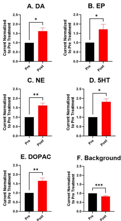
**Fig. 4** Statistics on current pre- and post-KOH treatment for each neurotransmitter on a CFME. Paired *t*-tests were performed for each analyte, normalized to pre-treatment (1),  $n = 6$ . (A)  $1 \mu\text{M}$  DA ( $p < 0.05$ ), (B)  $1 \mu\text{M}$  EP ( $p < 0.05$ ), (C)  $1 \mu\text{M}$  NE ( $p < 0.01$ ), (D)  $1 \mu\text{M}$  5-HT ( $p < 0.05$ ), (E)  $20 \mu\text{M}$  DOPAC ( $p < 0.01$ ), and (F) background ( $p < 0.001$ ).
