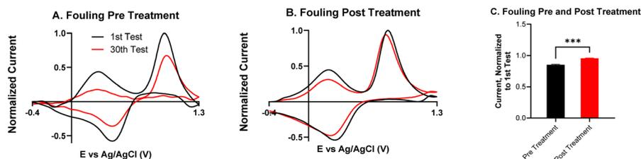
**Fig. 7** Electrode fouling measurements at an untreated and a KOH treated CNTYME.  $1 \mu\text{M}$  5-HT was injected for 5 seconds every 30 seconds, repeated 30 times. (A) CVs from an untreated CNTYME show a decrease on the 30th injection. (B) CVs from a 1-minute KOH treated CNTYME show the signal is largely preserved on the 30th injection. (C) Unpaired *t*-tests compare the 1st and 30th signal ( $p < 0.001$ ,  $n = 4$ ) and there was a significant difference in the fouling.
