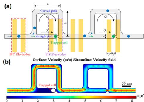
**Fig. 22** (a) The schematic representation of the microstructure combining electrical impedance spectroscopy and impedance flow cytometry shows the cell flowing or trapping. (b) The variability of flow velocity within the channels from an overhead perspective. Reproduced from ref. 202. Copyright 2019 American Chemical Society; permission obtained through Copyright Clearance Center, Inc.
