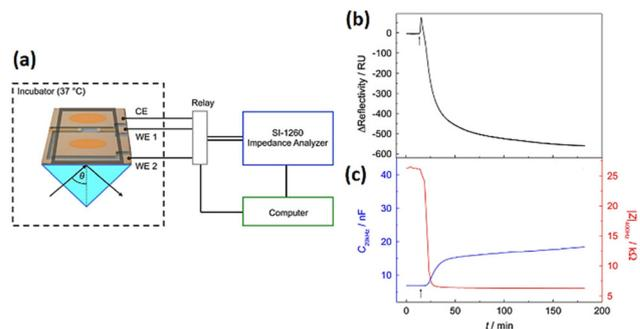
**Fig. 20** (a) Innovative arrangement for conducting simultaneous SPR and cell-based impedance analysis (b and c) The effect of 5  $\mu\text{M}$  cytochalasin D on a confluent MDCKII cell layer was measured using both SPR and ECIS techniques at the same time. The displayed content reproduced from ref. 183. Copyright 2013 Elsevier; permission obtained through Copyright Clearance Center, Inc.
