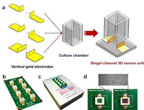
**Fig. 18** (a) An impedance biosensor design for three dimensions cell culturing. (b) Illustration of a three-dimensional impedance biosensor with eight channels. (c) Images of monitoring system. (d) Photographs taken of the platform both before and after it was seeded with live cells. The displayed content reproduced from ref. 166. Copyright 2019 Elsevier; permission obtained through Copyright Clearance Center, Inc.
