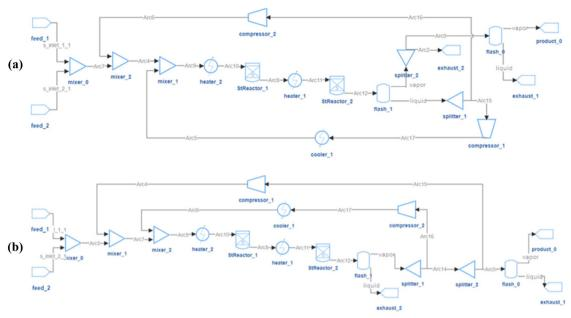
Fig. 11 Optimal flowsheets for HDA system with 20 units in pool. (a) product purity = 99.9%, product flow rate = 0.240 mol s<sup>-1</sup>; (b) product purity = 95.9%, product flow rate =  $0.288 \text{ mol s}^{-1}$
