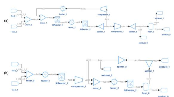
Fig. 14 Optimal flowsheets for methanol system with 18 units in pool. (a) product flow rate = 0.892 mol s<sup>-1</sup>, cost per mole product = 0.035 \$ per mol; (b) product flow rate =  $0.979 \text{ mol s}^{-1}$ , cost per mole product = 0.051\$ per mol.
