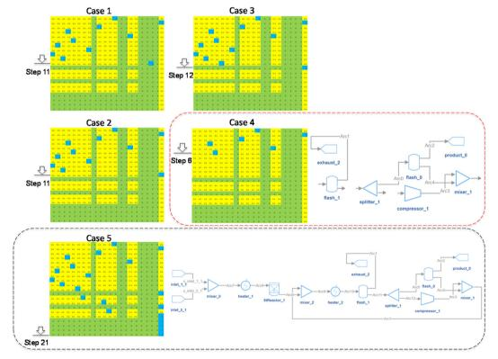
Fig. 8 Five kinds of actions. Case 1: 'inactive' action; Case 2: 'no action' with 'active' options; Case 3: 'no action' without 'active' options; Case 4: 'active' action; Case 5: episode end action.
