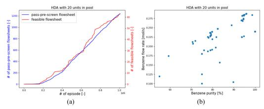
Fig. 10 RL results for HDA system with 20 units in pool. (a) the number of flowsheets founds within 1 million episodes; (b) the benzene flow rate and Benzene purity of the 64 feasible flowsheets for HDA-20.
