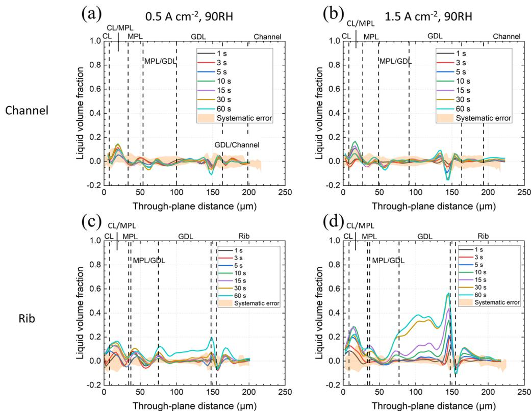
Fig. 3 Average liquid volume fraction (LVF) of product water in the CL, MPL and GDL of the *operando* VGCF-cell with 90% RH feed gases; LVF profiles are given at indicated times after the start of constant current operation with the estimated non-random error plotted as orange shade at (a) and (b)  $0.5 \text{ A cm}^{-2}$  &  $1.5 \text{ A cm}^{-2}$  under the channel, (c) and (d)  $0.5 \text{ A cm}^{-2}$  &  $1.5 \text{ A cm}^{-2}$  under the rib.
