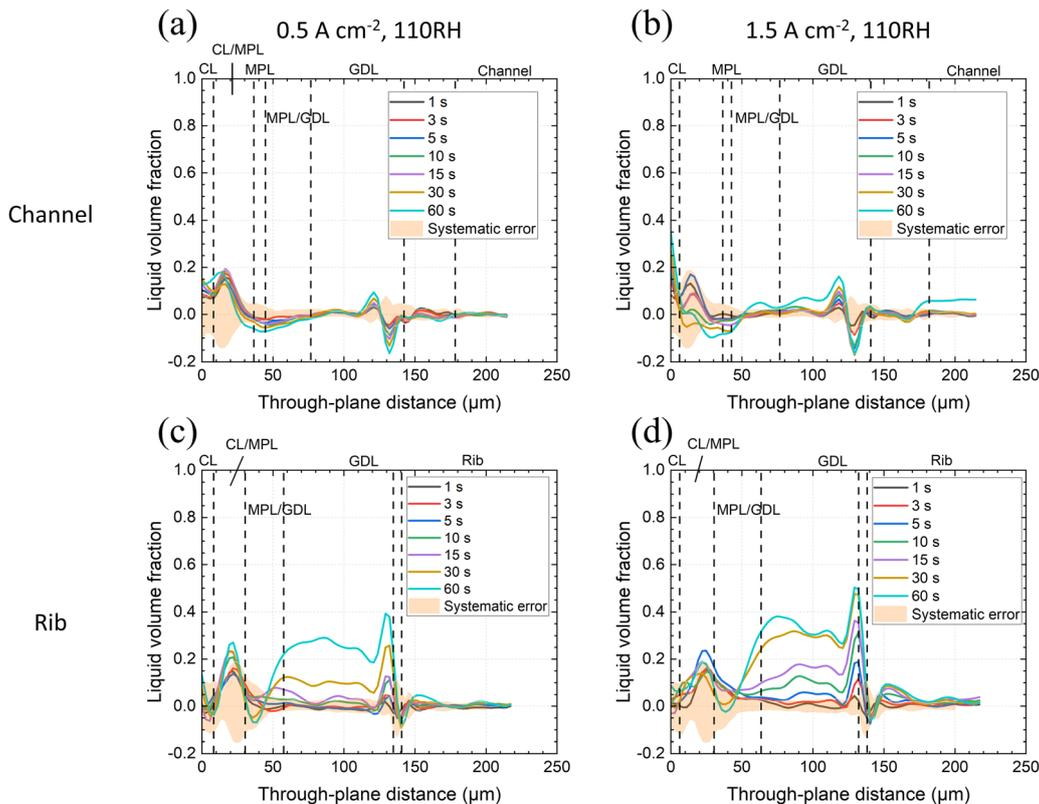
Fig. 7 Average liquid volume fraction (LVF) of product water in CL, MPL and GDL of the *operando* Li100-cell with 110% RH feed gases; LVF profiles are given at indicated times after the start of constant current operation are given with estimated non-random error plotted as orange shade at (a) and (b)  $0.5 \text{ A cm}^{-2}$  &  $1.5 \text{ A cm}^{-2}$  under the channel, (c) and (d)  $0.5 \text{ A cm}^{-2}$  &  $1.5 \text{ A cm}^{-2}$  under the rib.
