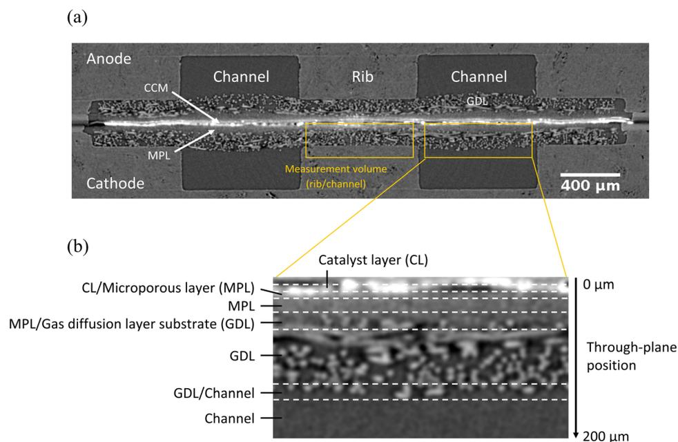
**Fig. 1** (a) X-ray tomographic through-plane image slice showing the components of the PEFC with Freudenberg H14 GDLs and VGCF MPL coating; (b) enlarged image under the channel region illustrating the different zones (CL, CL/MPL, MPL, MPL/GDL, GDL, GDL/Channel and Channel) of the PEFC for measurements (cathode). Dashed lines indicate that the zone boundaries are not always clear-cut.
