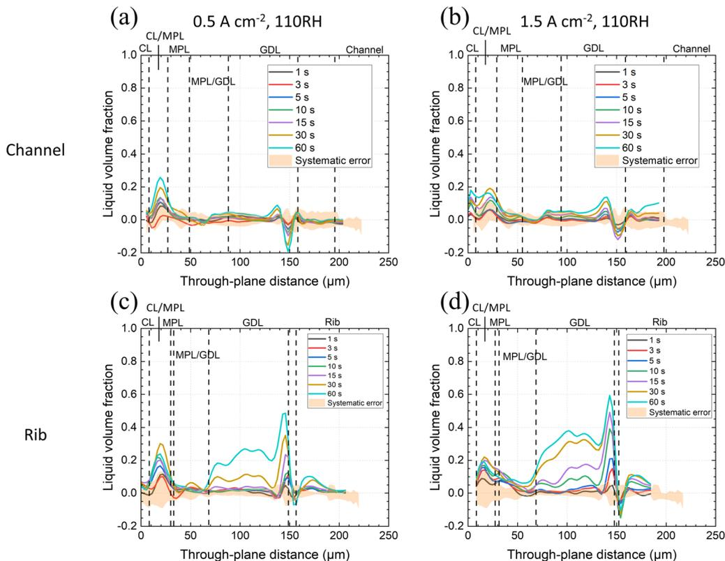
Fig. 4 Average liquid volume fraction (LVF) of product water in CL, MPL and GDL of the *operando* VGCF-cell with 110% RH feed gases; LVF profiles are given at indicated times after the start of constant current operation are given with estimated non-random error plotted as orange shade at (a) and (b)  $0.5 \text{ A cm}^{-2}$  &  $1.5 \text{ A cm}^{-2}$  under the channel, (c) and (d)  $0.5 \text{ A cm}^{-2}$  &  $1.5 \text{ A cm}^{-2}$  under the rib.
