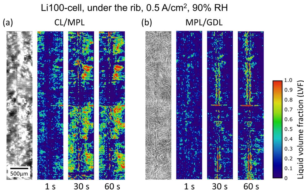
**Fig. 8** Liquid water distribution under the rib: (a) at the CL/MPL interface and (b) at the MPL/GDL interface of the Li100-cell operated at 0.5 A cm<sup>-2</sup>, 90% RH; from left to right: dry state tomographic image, product water LVF distribution maps at 1, 30 and 60 s PEFC operation time. The Li-100 LVF distribution maps are more susceptible to artifacts (horizontal lines) than the VGCF ones, due to more difficult registration.
