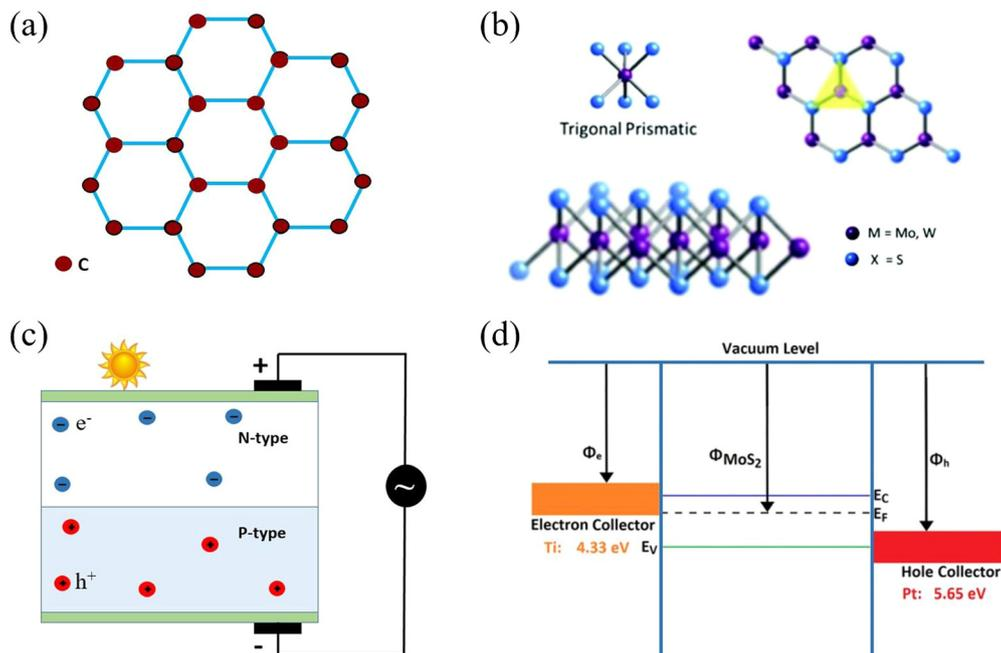
Fig. 3 (a) Honeycomb hexagonal structure of graphene. (b) Structure of 2D materials in terms of the metal coordination (top), and stacking sequence (bottom) of 2H MoS<sub>2</sub> and WS<sub>2</sub>. (c) Working principle of a photovoltaic cell (reprinted under Open Access<sup>51</sup>). (d) Schematic diagram in terms of the band structure of a Schottky junction Ti–MoS<sub>2</sub>–Pt solar cell (reprinted from ref. 52 under a CC-BY license).
