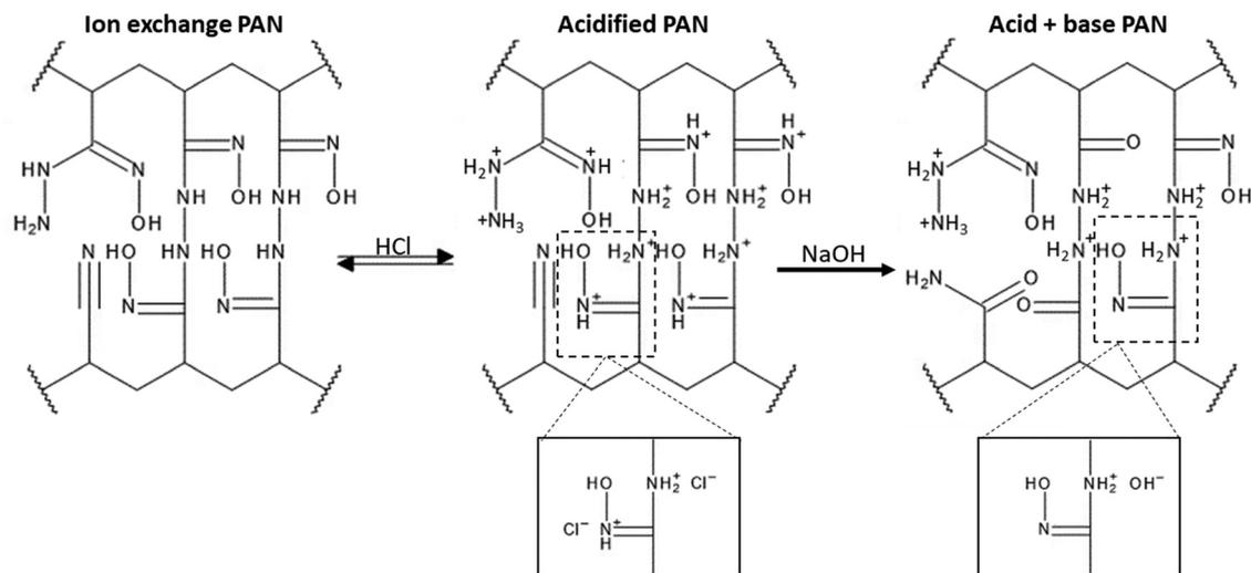
Scheme 1 Structures of the ion exchange PAN upon acidification and subsequent basification (Partially reproduced from Ahmed R.)<sup>23</sup>
