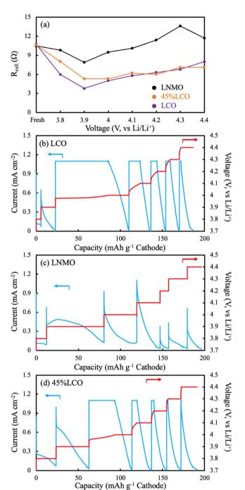
Fig. 7 (a) R<sub>cell</sub> as a function of voltage for AAM LNMO (black), AAM 45%LCO (orange), and AAM LCO (purple). Values were obtained by fitting EIS Nyquist plots. EIS was conducted after the voltage hold step of a CCCV chare of a cell with the indicated cathode paired with a lithium metal anode. The CCCV charge outcomes are displayed for the relevant cells with (b) LCO, (c) LNMO, and (d) 45%LCO, where red and blue curves represent the voltage and the current density, respectively.
