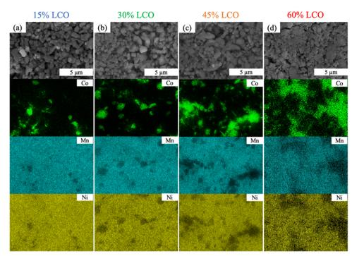
Fig. 2 SEM images (first row) and EDS maps (second, third, and fourth row) from AAM electrode cathodes of (a) 15%LCO, (b) 30%LCO, (c) 45%LCO, and (d) 60%LCO. The EDS maps correspond to the same regions as the SEM images and the color scale corresponds to locations where the indicated elements were detected: green for Co (second row), blue for Mn (third row), and yellow for Ni (fourth row)
