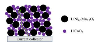
Fig. 1 Cartoon illustrating the LiCoO<sub>2</sub> (LCO) network in a multicomponent AAM electrode facilitating electronic conductivity through the electrode matrix. Larger black dots and smaller purple dots represent the LiNi<sub>0.5</sub>Mn<sub>0.5</sub>O2 (LNMO) and LCO particles, respectively. The green line depicts a relatively low resistance electronic conduction path from the current collector to a LNMO particle far from the current collector via the LCO network in the AAM electrode.
