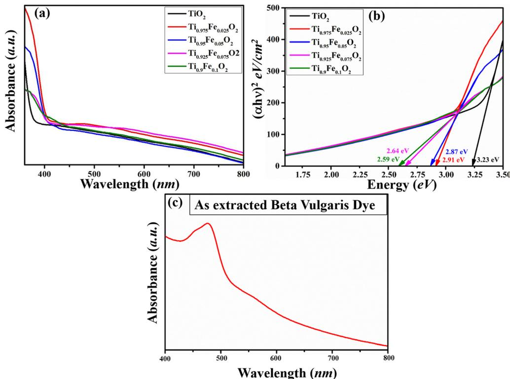
Fig. 6 Absorption spectra of (a)  $\text{Ti}_{1-x}\text{Fe}_x\text{O}_2$  ( $x = 0-0.1$ ) NRs, (b) Tauc plot of the  $\text{Ti}_{1-x}\text{Fe}_x\text{O}_2$  ( $x = 0-0.1$ ) NRs and (c) UV-Visible spectra of the extracted BV dye.
