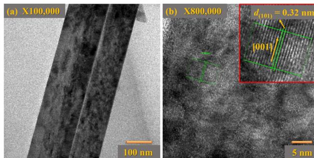
Fig. 4 (a) TEM images of a single  $\text{TiO}_2$  NR, and (b) the corresponding HRTEM image of a single  $\text{TiO}_2$  NR. The inset image of (b) displays the lattice spacing between (101) planes of rutile phase  $\text{TiO}_2$ .
