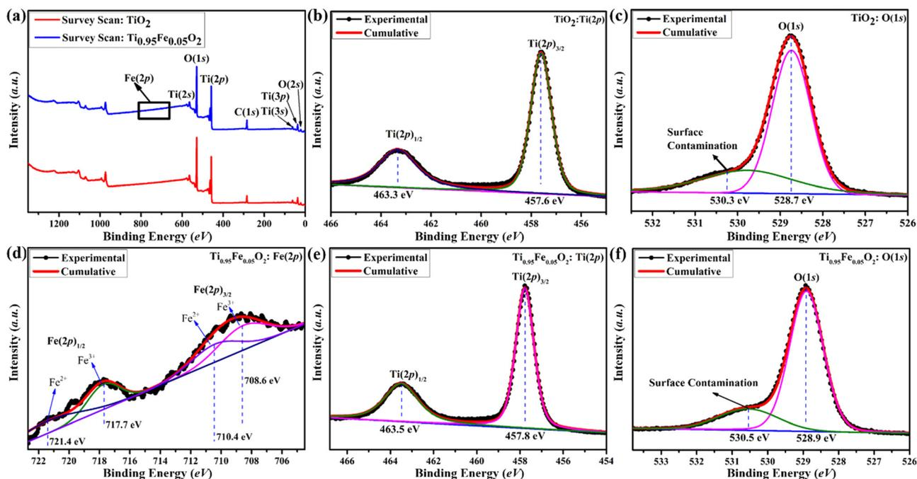
Fig. 5 The XPS spectra of bare  $\text{TiO}_2$  and  $\text{Ti}_{0.95}\text{Fe}_{0.05}\text{O}_2$  photoanodes. (a) Comparison of XPS survey scan spectra, (b)  $\text{TiO}_2$ : Ti(2p) core-level XPS spectra, (c)  $\text{TiO}_2$ : O(1s) core-level XPS spectra, (d)  $\text{Ti}_{0.95}\text{Fe}_{0.05}\text{O}_2$ : Fe(2p) XPS spectra, (e)  $\text{Ti}_{0.95}\text{Fe}_{0.05}\text{O}_2$ : Ti(2p) core-level XPS spectra, and (f)  $\text{Ti}_{0.95}\text{Fe}_{0.05}\text{O}_2$ : O(1s) core-level XPS spectra.
