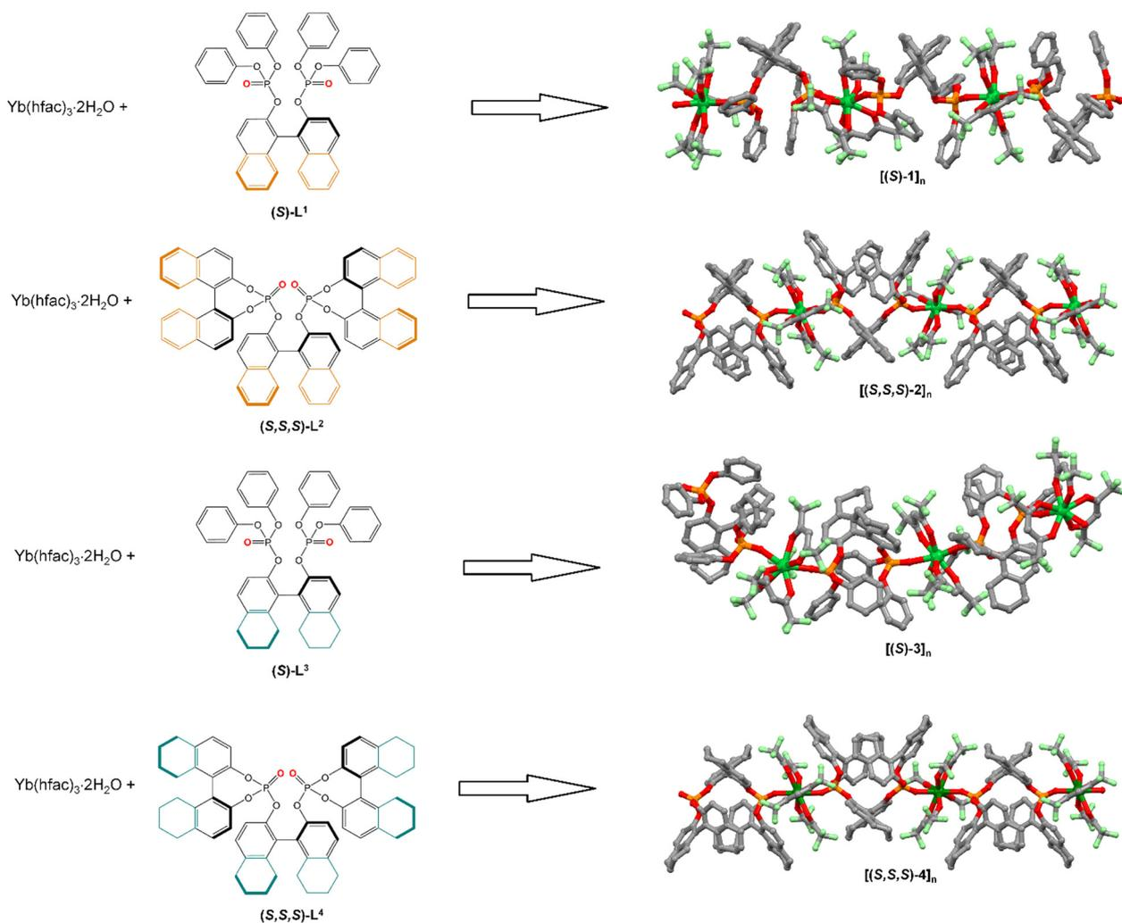
**Scheme 1** Coordination reactions of the formation of  $[(S)-1]_n$ ,  $[(S,S,S)-2]_n$ ,  $[(S)-3]_n$  and  $[(S,S,S)-4]_n$  polymers with molecular structures of the (S)-enantiomer of the four ligands emphasizing the difference between the ligands. The  $[(S,S,S)-4]_n$  drawing was made from the X-ray structure of the dysprosium analogue.
