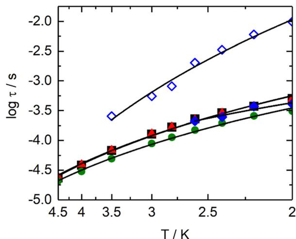
Fig. 3 Temperature variations in the relaxation times in the range of 2–4.5 K under 1000 Oe for [(S)-1]<sub>n</sub> (full black squares), [(S,S,S)-2]<sub>n</sub> (full blue lozenges for LF contribution and empty blue lozenges for HF contribution), [(S)-3]<sub>n</sub> (full red up-triangles) and [(S,S,S)-4]<sub>n</sub> (full green circles). The black lines depict the best fits with the parameters given in the text.
