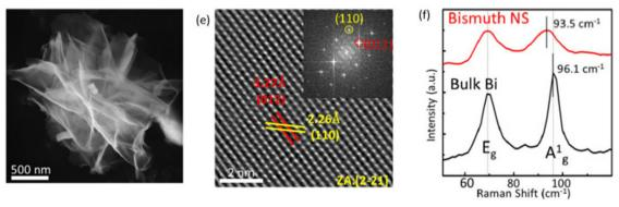
Fig. 5 (a) TEM image, (b) HRTEM image and (c) Raman spectra of bismuthene nanosheets. Reprinted with permission from Wiley.<sup>57</sup>
