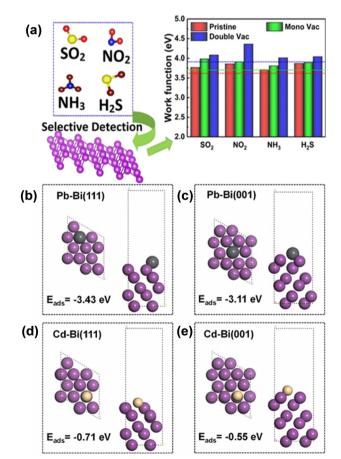
Fig. 7 (a) Sensing of SO<sub>2</sub>, NO<sub>2</sub>, NH<sub>3</sub>, and H<sub>2</sub>S gas using bismuthene. Reprinted with permission from ACS. 85 Adsorption energies and adsorption configurations of lead on (b) Bi-ene and bismuth nanosheets (c) and cadmium on Bi-ene (d) and (e) bismuth nanosheets, respectively (black, yellow and violet balls represent Pb, Cd and Bi atoms, respectively) Reprinted with permission from Elsevier.86
