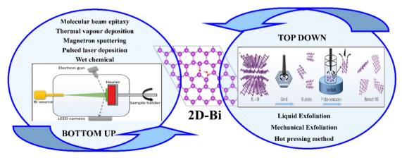
Fig. 6 Schematic representation of the different techniques for the synthesis of monoelemental bismuthine
