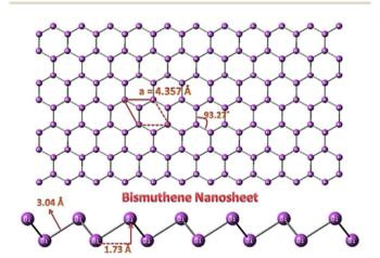
Fig. 1 Schematic of bismuthene nanosheet. Reprinted with permission from Elsevier.<sup>13</sup>
