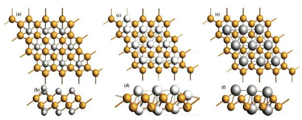
Fig. 11 Fully lithiated, sodiated and potassiated b-Bi structures from z-axis (a, c and e) and x-axis (b, d and f) views, respectively. Reprinted with permission from Elsevier. 108
