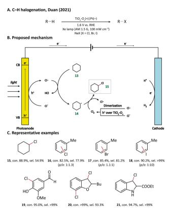
Photoanode-mediated cyclohexane halogenation.
