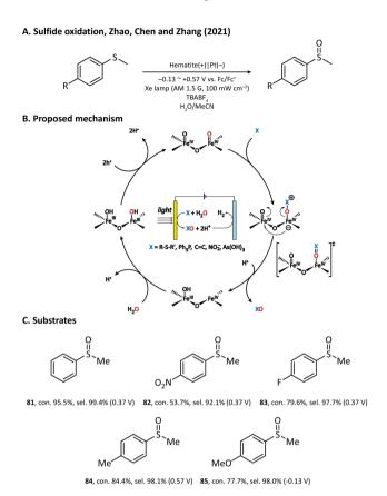
Fig. 12 Hematite-mediated oxygen atom transfer reaction.
