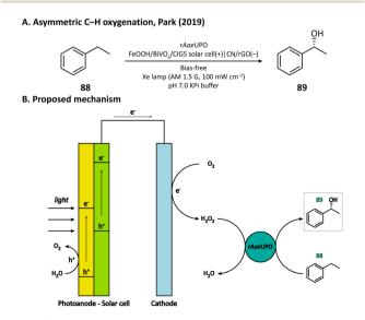
Fig. 14 Cathode-mediated in situ  $H_2O_2$  generation for asymmetric C-H oxygenation.
