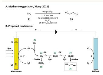
Photoanode-mediated methane oxygenation.
