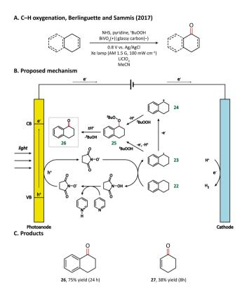
Fig. 4 Photoanode-mediated C-H oxygenation at the  $\alpha$ -position of the alkane and arene
