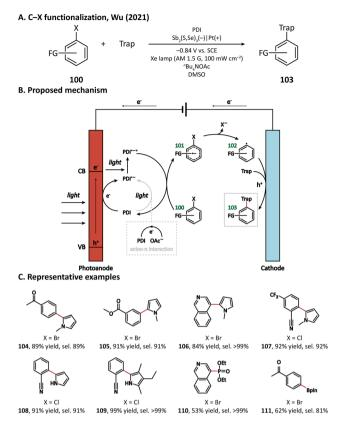
Fig. 18 Photocathode-mediated C-X activation
