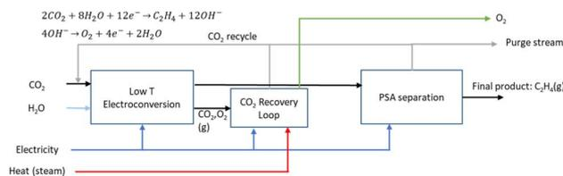
**Fig. 9** Process diagram of the LT CO<sub>2</sub> electrolysis towards C<sub>2</sub>H<sub>4</sub>.
