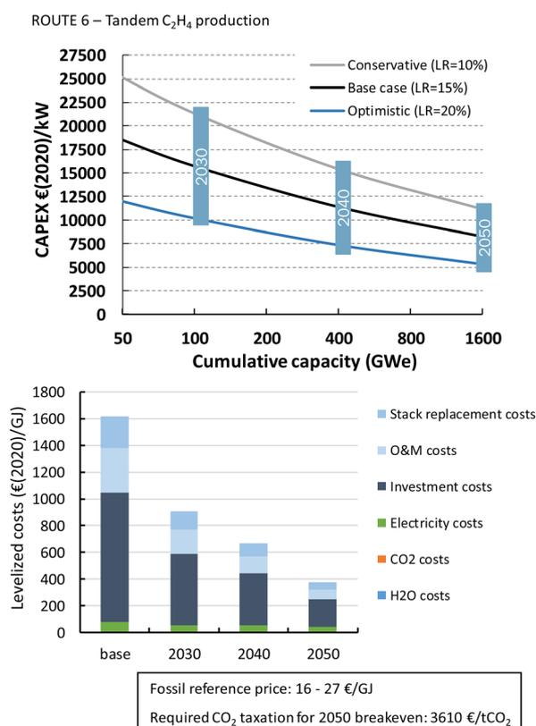
Fig. 30 Route 6 cost projections of the CAPEX (top) and the base case levelized C<sub>2</sub>H<sub>4</sub> production costs (bottom) for Tandem electrochemical CO<sub>2</sub> conversion to ethylene. The CIC of LT electroconversion processes in 2020 is 45 GWe.
