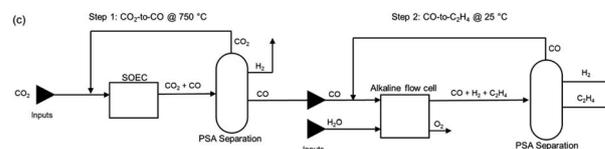
Fig. 19 Process diagram of the tandem HT CO<sub>2</sub> electrolysis to CO and LT CO electrolysis towards C<sub>2</sub>H<sub>4</sub>, the so-called tandem process. Adapted from Sisler et al., 2021.<sup>51</sup>Table 14 Investment costs for the HT CO<sub>2</sub>-SOE plant to produce syngas
