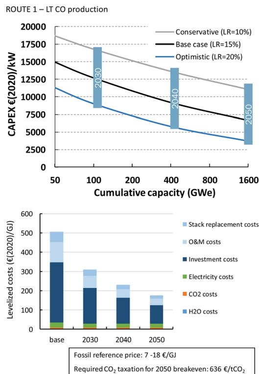
Fig. 25 Route 1 cost projections of the CAPEX (top) and the base case levelized CO production costs (bottom) for LT electrochemical CO<sub>2</sub> conversion to carbon monoxide. The CIC of LT electroconversion processes in 2020 is 45 GW<sub>e</sub>.
