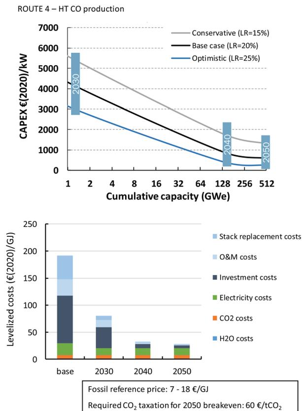
Fig. 28 Route 4 cost projections of the CAPEX (top) and the base case levelized CO production costs (bottom) for HT electrochemical CO<sub>2</sub> conversion to carbon monoxide. The CIC of HT electroconversion processes in 2020 is 0.5 GWe.
