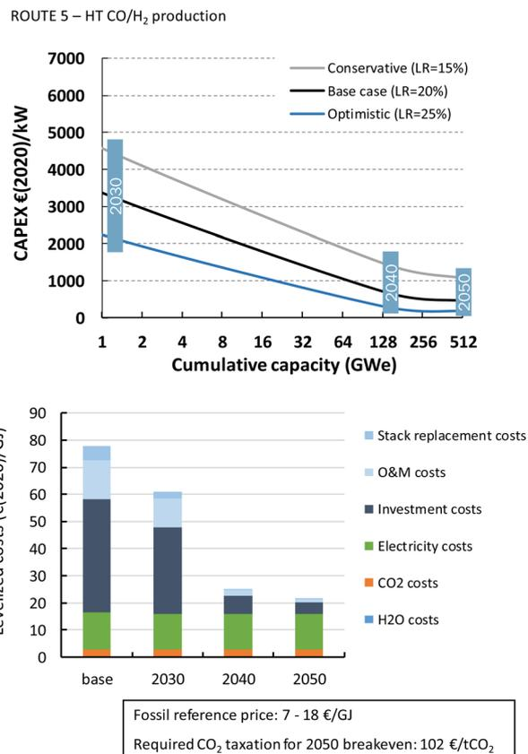
Fig. 29 Route 5 cost projections of the CAPEX (top) and the base case levelized syngas production costs (bottom) for HT electrochemical CO<sub>2</sub> conversion to syngas. The CIC of HT electroconversion processes in 2020 is 0.5 GWe.
