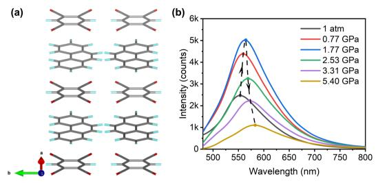
Fig. 5 (a) The sketch map for molecular packing of Phe-TCNB. (b) High-pressure PL spectra of Phe-TCNB.
