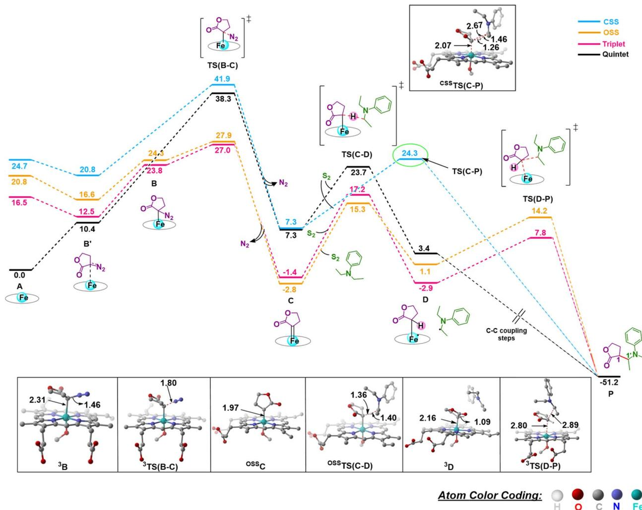
Fig. 1 Gibbs free energy profile (kcal mol<sup>-1</sup>) of N<sub>2</sub> extrusion and subsequent C–H insertion at different spin states of Fe. Distances are in Å. The H atoms are omitted for clarity.
