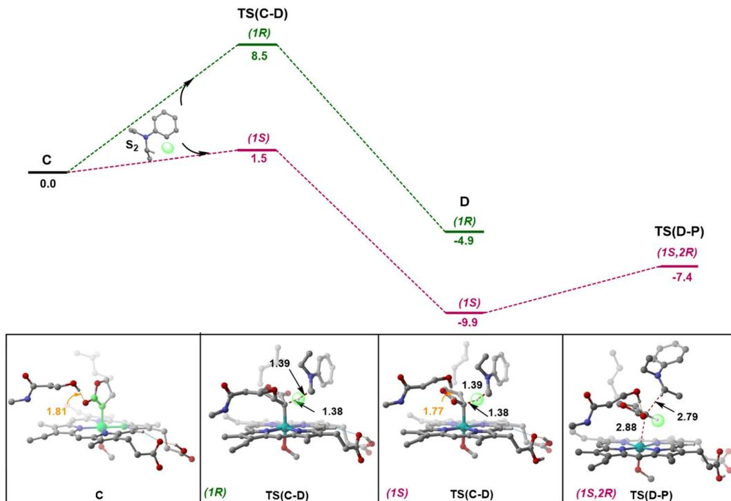
Fig. 6 Total electronic energy profile of L9 ( $\text{kcal mol}^{-1}$ ) for HAT and the lowest-energy radical rebound TSs with  $\text{S}_2$  approaching from face A are shown. The H atoms (except the ones taking part in H-bonding) are omitted for clarity.
