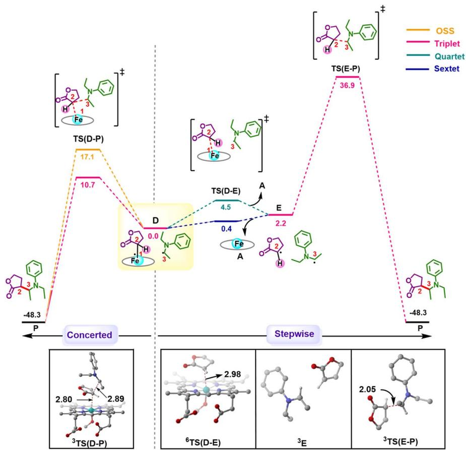
Fig. 2 Gibbs free energy profile ( $\text{kcal mol}^{-1}$ ) for comparison of concerted and stepwise pathways for C–H insertion at different spin states of Fe. Distances are in Å. The H atoms are omitted for clarity.
