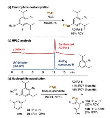
Fig. 2 (a) Electrophilic destannylation of tributyltin precursor 7 with At $^+$  species gave ADIPA 6 in 88% RCY. (b) HPLC analysis of synthesized ADIPA 6 (red line, monitored by the  $\gamma$  detector) and analog compound 8 (blue line, monitored by UV detector at 254 nm) shows identical retention time (12 minutes). (c) Nucleophilic substitution of aryliodonium salts 9a or 9b with At $^-$  species gave ADIPA 6 and side products 10a or 10b, respectively.
