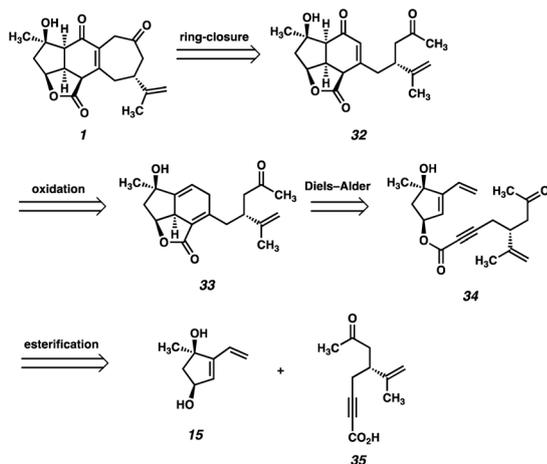
Fig. 3 Second-generation retrosynthetic analysis of scabrolide A (1).
