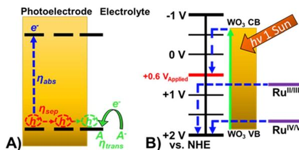
Fig. 4 (A) Schematic of oxidation occurring at a photoelectrode demonstrating the efficiencies that govern observed photocurrent. (B) Energy diagram of Ru-UiO-67/WO<sub>3</sub> at pH 6.
