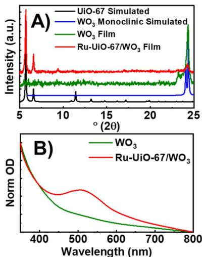
Fig. 1 (A) PXRD patterns of simulated UiO-67 (black), monoclinic  $\text{WO}_3$  (red),  $\text{WO}_3$  film (blue), and Ru-UiO-67/ $\text{WO}_3$  (orange). (B) Ground-state absorption spectra of  $\text{WO}_3$  (black), and Ru-UiO-67/ $\text{WO}_3$  (red).
