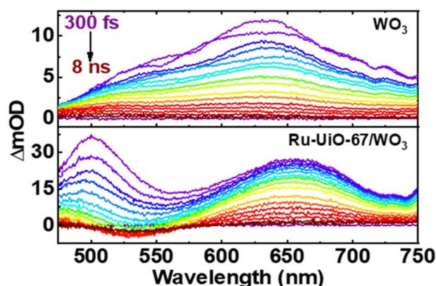
Fig. 6 Ultrafast transient absorption spectral mappings (purple to red) of  $WO_3$  (top) and  $Ru-Uio-67/WO_3$  (bottom) films on glass under an Ar atmosphere.  $\lambda_{ex}$  = 320 nm,  $\sim 200 \mu J cm^{-2}$ .
