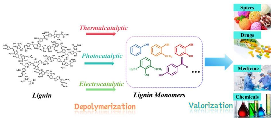
Fig. 1 Catalytic lignin depolymerization pathways for utilization.
