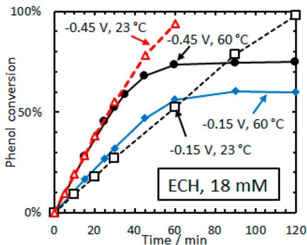
Fig. 15 Conversion versus time for ECH of phenol (18 mM) on 5 wt% Rh/C in aqueous acetate buffer. Adapted from ref. 36 with permission. Copyright 2016 American Chemical Society.
