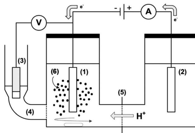
Fig. 14 A sketch of electrochemical cell setup (H-cell) for ECH of guaiacol and phenol: (1) cathode, (2) anode, (3) reference electrode (Ag/AgCl/3 M KCl), (4) fritted side compartment (Luggin probe) for reference electrode filled with 3 M KCl, (5) cation exchange membrane, and (6) catalyst slurry. Adapted from ref. 33 with permission. Copyright 2019 Wiley-VCH.
