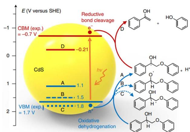
Fig. 9 Potentials of oxidative dehydrogenation of PP-ol via three different paths (A, B, C) and potential of reductive cleavage of  $\beta$ -O-4 bond in the  $C_\alpha$  radical intermediate (D) against the positions of VBM and CBM of CdS. Experimental values of VBM and CBM were obtained through UV-visible and electrochemical measurements of bulk CdS. Adapted from ref. 20 with permission. Copyright 2018 Springer Nature.
