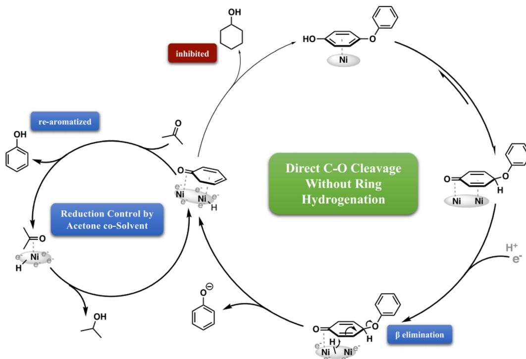
Fig. 16 Selective inhibition of aromatic ring reduction by acetone co-solvent. Schematic illustration of product selectivity control by the inclusion of acetone as a co-solvent during ECH of 4-phenoxyphenol. Adapted from ref. 38 with permission. Copyright 2022 Springer Nature.
