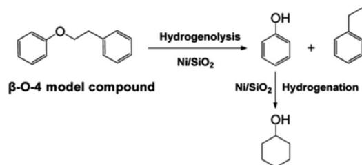
Fig. 4 Reaction pathway for the cleavage of 2-phenylethyl phenyl ether (the model compound for the  $\beta$ -O-4 linkage in lignin) over Ni/SiO<sub>2</sub> in the aqueous phase. Adapted from ref. 8 with permission. Copyright 2012 American Chemical Society.
