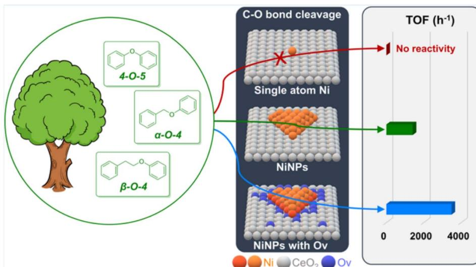
Fig. 7 Comparison of catalyst activity of different sizes. Adapted from ref. 17 with permission. Copyright 2023 American Chemical Society.
