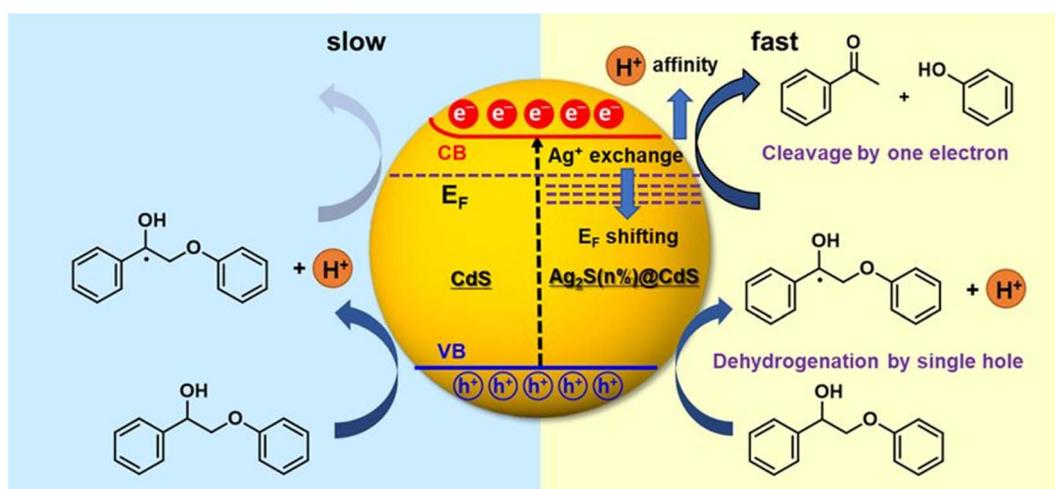
**Fig. 11** Schematic representation comparing the simultaneous oxidative dehydrogenation and reductive cleavage of the  $\beta\text{-O-4}$  bond in the  $\text{C}_\alpha$  radical intermediate in  $\text{Ag}_2\text{S}@\text{CdS}$  (right) with the oxidative dehydrogenation and pinned Fermi level of CdS (left). Adapted from ref. 22 with permission. Copyright 2020 American Chemical Society.
