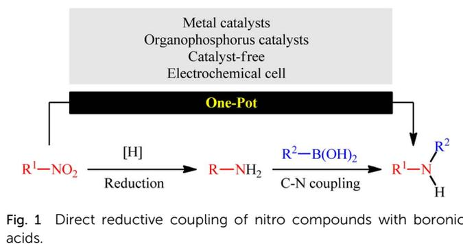
Fig. 1 Direct reductive coupling of nitro compounds with boronic acids.
