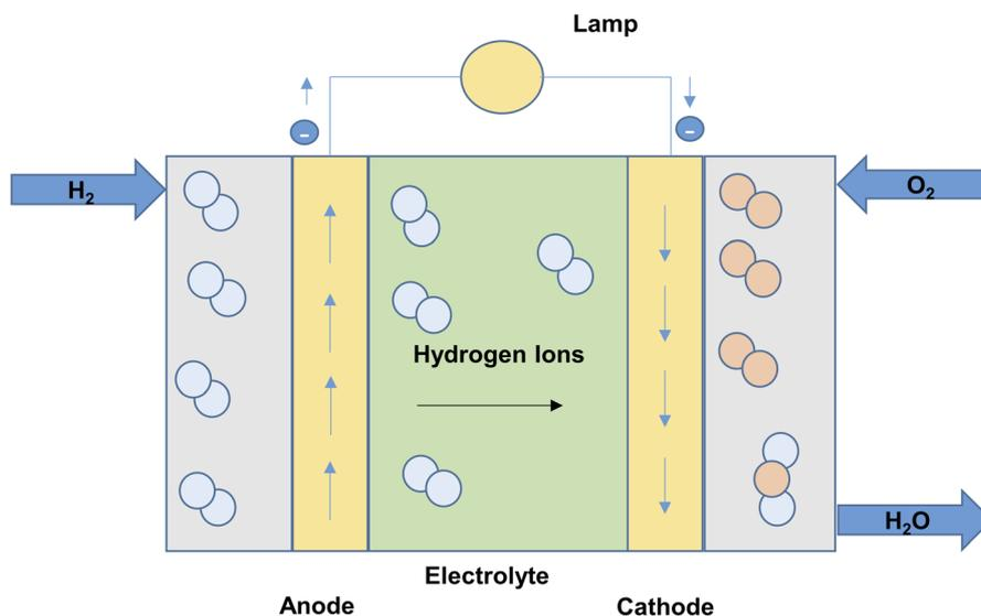
Fig. 13 A schematic of PAFC.
