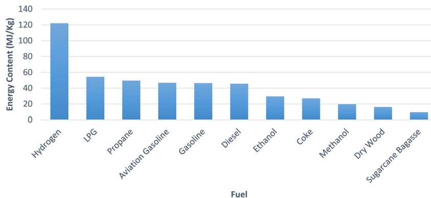
Fig. 1 Energy content of different fuels (drawn using data from ref. 6).
