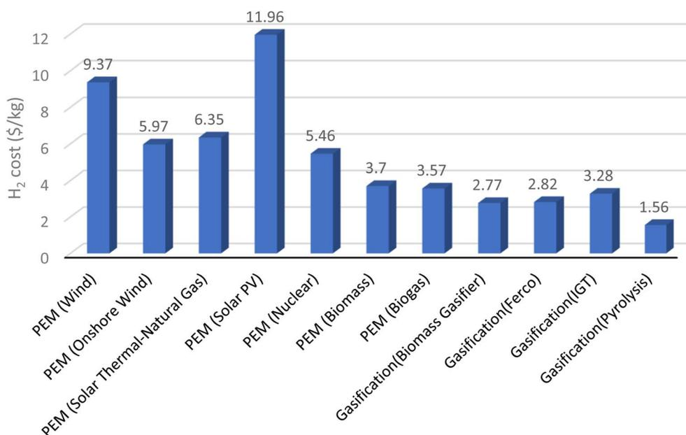
Fig. 15 Hydrogen production costs associated with different technologies.
