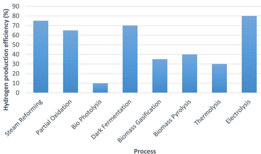
Fig. 9 Hydrogen production efficiency of different processes.
