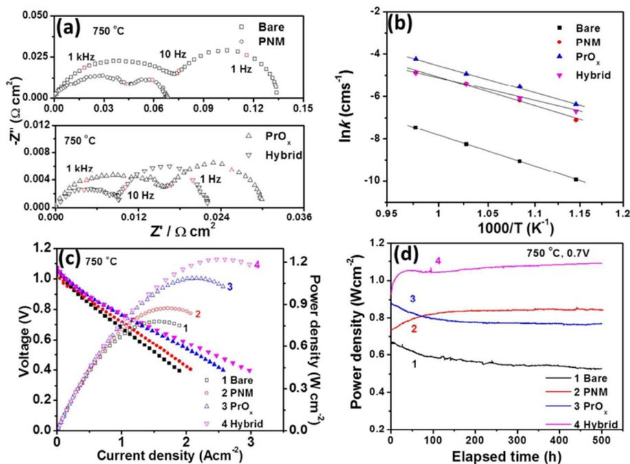
Fig. 20 (a) Impedance spectroscopy of bare cathode and PNM cathode (b) conductivity plot (c)  $I$ - $V$  curves (d) peak power density over time. (Reproduced with permission from ref. 114 Copyright 2017 Royal Society of Chemistry.)
