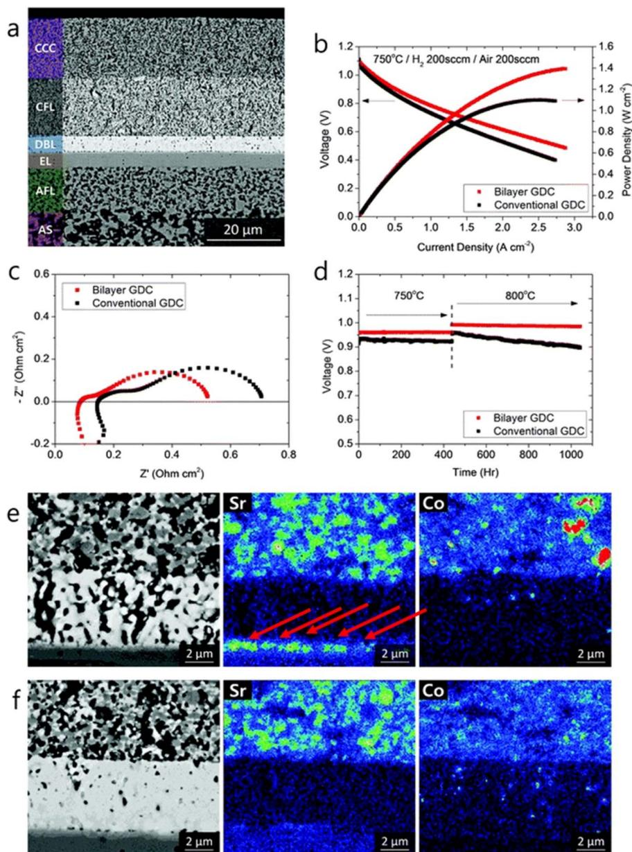
Fig. 15 (a) Microstructure of anode-supported cell with bilayer GDC (b)  $I$ - $V$  curves, (c) impedance spectra and (d) long-term evaluation results of the cells with bilayer and conventional GDC. (e) Post-test EDS analysis of conventional cell. (f) Post-test EDS analysis of bilayer cell. (Reproduced with permission from ref. 32 Copyright 2018 Royal Society of Chemistry.)
