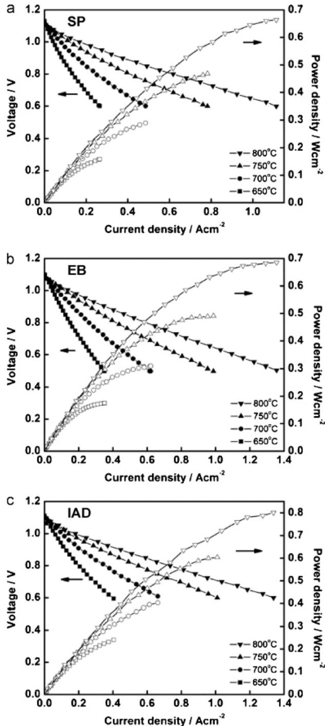
Fig. 34  $I$ - $V$  curves of cells fabricated from GDC deposited by (a) screen printing (b) electron beam evaporation (c) ion assisted deposition. Reproduced with permission from ref. 85 Copyright 2011 Elsevier.
