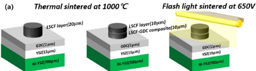
Fig. 16 (a) Anode supported LSCF–GDC cathode cell configuration, and flashlight sintering process. (Reproduced with permission from ref. 54 Copyright 2022 Elsevier.)
