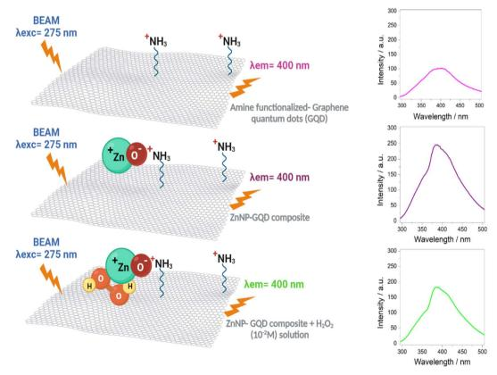
Fig. 9 Reaction scheme for the H<sub>2</sub>O<sub>2</sub> detection in the ZD1-t sample shown in the Fig. 5d.
