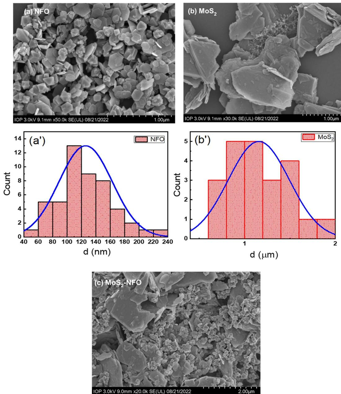
Fig. 2 (a–c) SEM images of the as-synthesized materials (NFO, MoS<sub>2</sub>, and MoS<sub>2</sub>-NFO); (a' and b') size distribution of NFO and MoS<sub>2</sub> samples.
