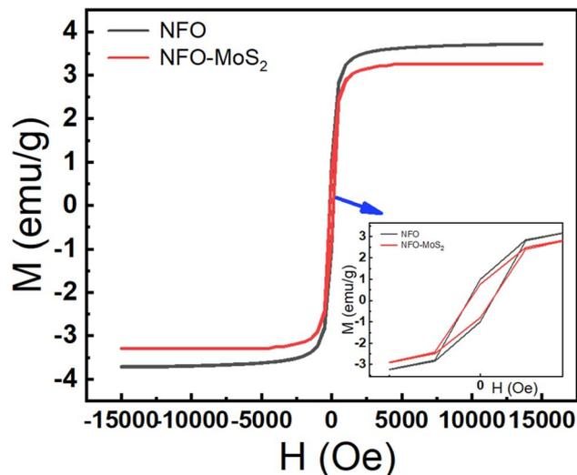
Fig. 3 Magnetization curves of NFO and MoS<sub>2</sub>-NFO samples.
