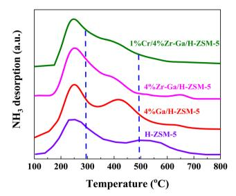
Fig. 2  $NH_3$ -TPD profiles of the bare and Ga-, Zr-Ga-, and Cr/Zr-Ga-doped H-ZSM-5.
