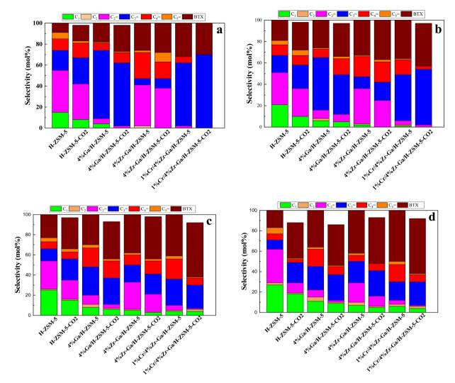
Fig. 7 Product distribution of bare and metal-doped H-ZSM-5 zeolites at (a) 400 °C, (b) 450 °C, (c) 500 °C, and (d) 550 °C. Reaction conditions: pressure, 1 bar; feed gas,  $C_3H_8/N_2 = 2.5/97.5$  and  $C_3H_8/CO_2/N_2 = 2.5/5/92.5$ ; flow rate, 75 mL min<sup>-1</sup>; WHSV, 4 kg<sub>cat</sub> s mol<sub>C,H<sub>s</sub></sub><sup>-1</sup>.
