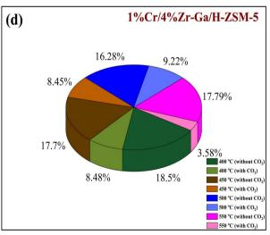
Fig. 8 Deactivation factor of the bare and metal-doped H-ZSM-5 zeolites at (a) 400 °C, (b) 450 °C, (c) 500 °C, and (d) 550 °C. Reaction conditions: pressure, 1 bar; feed gas,  $C_3H_8/N_2=2.5/97.5$  and  $C_3H_8/CO_2/N_2=2.5/5/92.5$ ; flow rate, 75 mL min<sup>-1</sup>; WHSV, 4 kg<sub>cat</sub> s mol<sub>C3H8</sub><sup>-1</sup>.
