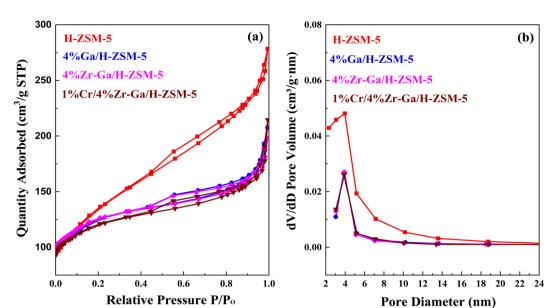
Fig. 4 (a) N<sub>2</sub> physisorption isotherm and (b) the BJH pore size distributions.
