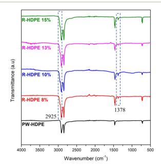
Fig. 2 FTIR spectra of the HDPE membranes.
