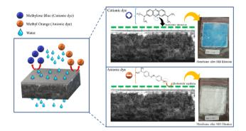
Fig. 10 Dye removal scheme.
