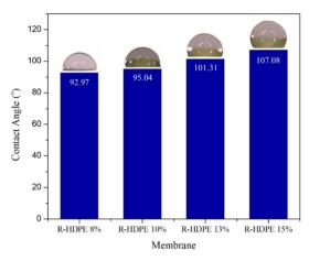
Fig. 5 Contact angles of the membranes.
