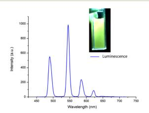
Fig. 4 The delayed luminescence spectra of  $[Tb(4)_3]^{3+}(2.7 \times 10^{-5} \text{ M})$  recorded in CH<sub>3</sub>CN showing the characteristic Tb(III) transitions  $^5D_4 \rightarrow ^7F_{6,5,4,3,2}$ . Inset: green Tb(III) emission that was visible to the naked eye upon placing the sample under a UV-Vis lamp.
