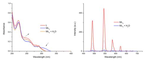
Fig. 8 (Left) Absorbance spectra of ligand 6 upon addition of Tb(|||) at 0 and 3 equivalents of Tb(|||), and upon addition of  $H_2O$ . (Right) the Tb(|||) emission spectrum of the 1:3 complex showing decrease in luminescence intensity upon the addition of  $H_2O$ .
