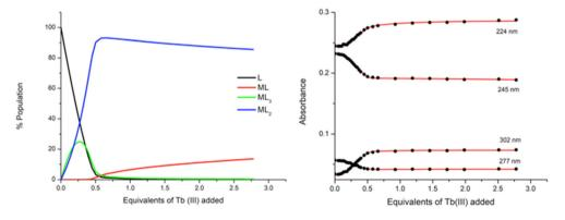
Fig. 7 (Left) the speciation distribution diagram obtained from the fit of the UV-visible absorption titration data of ligand 4 against Tb(CF<sub>3</sub>SO<sub>3</sub>)<sub>3</sub> in CH<sub>3</sub>CN. (Right) the fit of the experimental binding isotherms using non-linear regression analysis software ReactLab.
