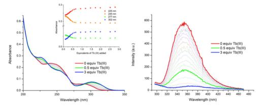
Fig. 5 The observed spectroscopic changes for 4 (1 × 10<sup>-5</sup> M) against Tb(CF<sub>3</sub>SO<sub>3</sub>)<sub>3</sub> (0 → 3 equiv.) in CH<sub>3</sub>CN at RT. (Left) the UV-visible absorption spectra. Inset: corresponding experimental binding isotherms with absorbance at  $\lambda = 225, 245, 277$  and 300 nm. (Right) the corresponding changes in the fluorescence emission spectra,  $\lambda_{ex}$  = 255 nm.
