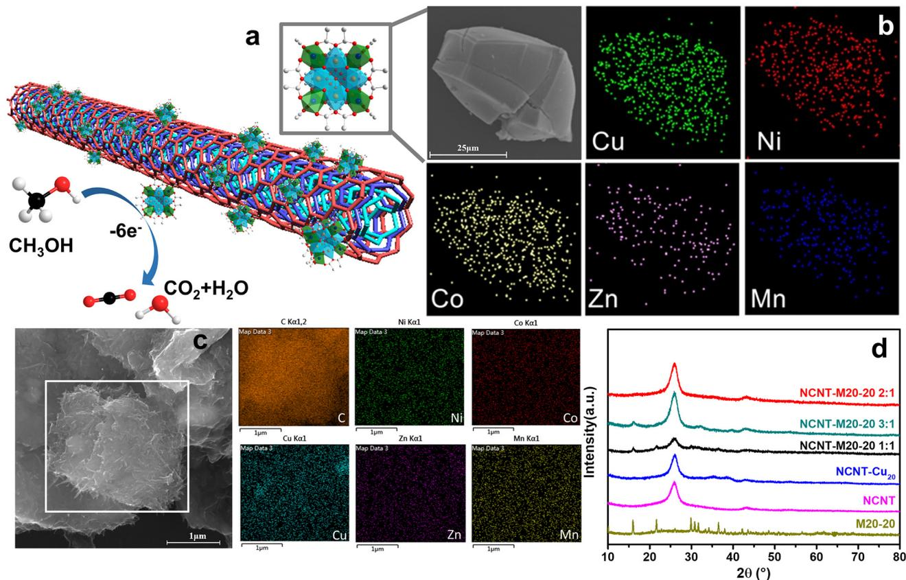
**Fig. 2** Structural characterizations of the NCNT-M20-20 composite. (a) Graphic illustration of NCNT-M20-20 2:1 in the MOR process, with the structure of M20-20 shown as a ball-and-stick model. (b) Morphology of M20-20 and mapping information of the selected area. (c) Morphology of NCNT-M20-20 2:1 and EDS results. (d) Powder XRD of a series of materials.
