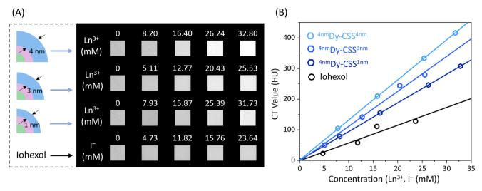
Fig. 4 (A) CT images of Cit-Dy-CSS (Cit-<sup>4nm</sup>Dy-CSS<sup>1nm</sup>, Cit-<sup>4nm</sup>Dy-CSS<sup>3nm</sup>, and Cit-<sup>4nm</sup>Dy-CSS<sup>4nm</sup>) NPs and clinically used CT CA iohexol at different concentrations. (B) CT values for different concentrations of Cit-Dy-CSS NPs dispersed in water and iohexol solutions. Solid lines are linear fits.
