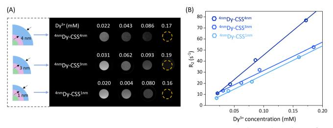
Fig. 3 (A)  $T_2$ -Weighted MR images of Cit-Dy-CSS NPs with varying NaDyF<sub>4</sub> outer shell thickness (Cit-<sup>4nm</sup>Dy-CSS<sup>3nm</sup>, Cit-<sup>4nm</sup>Dy-CSS<sup>3nm</sup> and Cit-<sup>4nm</sup>Dy-CSS<sup>4nm</sup>) as a function of the Dy<sup>3+</sup> concentration. (B) Relaxation rate  $R_2$  (=1/ $T_2$ ) of water protons plotted against the molar concentration of Dy<sup>3+</sup> at 7 T. Solid lines are linear fits.
