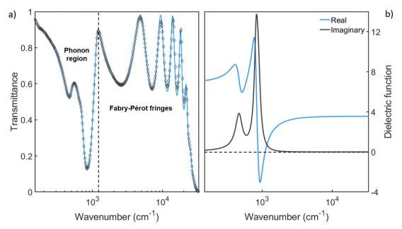
Fig. 1 (a) Experimental (light blu line) and fitted (black empty diamond symbols) transmittance of the Si<sub>3</sub>N<sub>4</sub> membrane, measured in the THz-UV range. The vertical black dashed line separates the phonon absorption region (low-frequency) to the high-frequency part characterized by Fabry-Pérot fringes. (b) Real (light blue line) and imaginary (black line) parts of the dielectric function, extracted from the fitted transmittance by considering the Fabry-Pérot effect.
