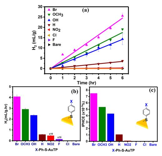
Fig. 3 (a) Photocatalytic  $H_2$  production observed over time for various X-Ph-S-AuTP substrates, (b) the  $H_2$  production rate, and (c) IPHCE calculated for each substrate. The experiment was performed in neutral water under 808 nm laser illumination with a power density of 100 mW cm<sup>-2</sup>.
