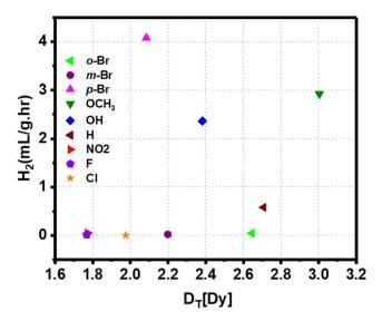
Fig. 5 Correlation between the dipole moment of the Au-ligand system for various substituents and hydrogen production rate.
