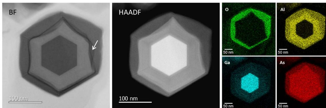
Fig. 8 Axial cross-sectional BF-STEM and HAADF-STEM images of another typical nanowire with EDS elemental mapping for O, Al, Ga, and As for the identical GaAs/Al<sub>0.8</sub>Ga<sub>0.2</sub>As core-shell nanowire sample shown in Fig. 2.
