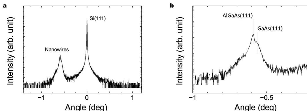
Fig. 6 (a)  $\theta$ – $2\theta$  XRD scan of the GaAs/Al<sub>0.8</sub>Ga<sub>0.2</sub>As core-shell nanowires investigated, and (b) enlarged curve for the peak originating from the nanowires. The centers of the curves were adjusted relative to the Si(111) reflection peak at  $14.22^\circ$ .
