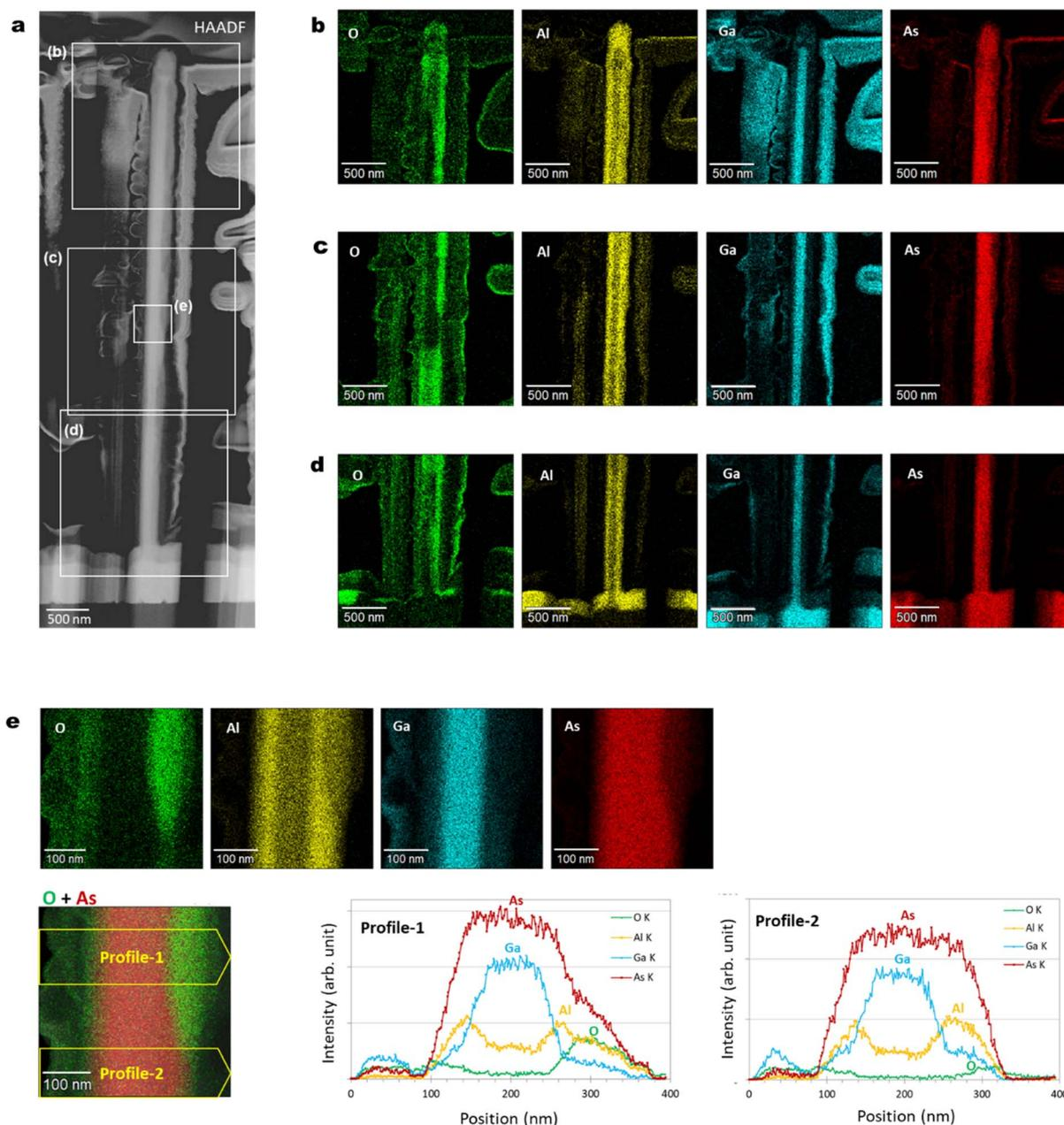
Fig. 10 (a) BF-STEM image, and (b)–(d) EDS elemental maps of O, Al, Ga, and As for the areas indicated by the squares in (a) for a single GaAs/Al<sub>0.8</sub>Ga<sub>0.2</sub>As core-shell nanowire. (e) Enlarged EDS elemental maps for the areas indicated by the squares in (a), and EDS elemental distributions along the profiles through the nanowire shown in the superimposed elemental maps for O and As in the bottom left panel.
