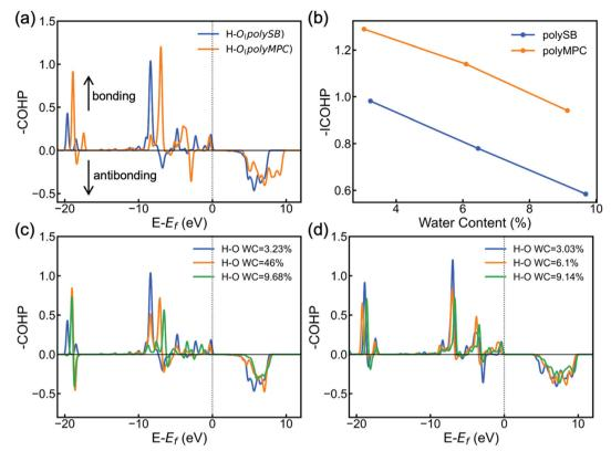
Fig. 5 (a) Crystal orbital Hamilton population (-COHP) of the bond between hydrogen atom of the adsorbed H<sub>2</sub>O and the nearest oxygen of polySB and polyMPC at WC = 3.23% and 3.03%, respectively. (b) Integrated -COHP (-ICOHP) vs. water content, calculated -COHP for the bond between hydrogen atom of adsorbed H<sub>2</sub>O and nearest oxygen atom of the polySB (c) and polyMPC (d) at different WC.
