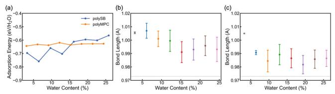
Fig. 3 (a) Calculated water adsorption energy per water molecule vs. WC. (b) and (c) The mean and standard of deviation of the Owater-H<sub>water</sub>···O<sub>poly</sub> covalent bond length in the adsorbed water molecules where the H<sub>water</sub> atom is bonded to O<sub>poly</sub> atom of polyMPC and polySB, respectively. The horizontal dashed line points to  $O_{water}$ - $H_{water}$  covalent bond length of 0.973 Å in free water molecule.
