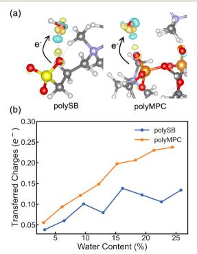
Fig. 4 (a) Differential charge density plots for both polymers with two adsorbed water molecules (yellow color: charge accumulation; cyan color: charge depletion). (b) Total charge transferred from polymers to the adsorbed water molecules based on Bader charges.
