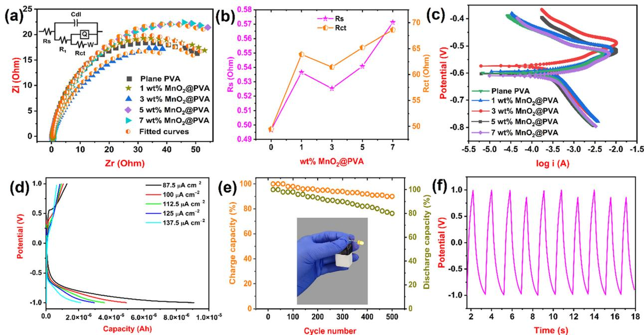
Fig. 4 (a) Nyquist plot of all gel electrolytes with an equivalent circuit. (b) Variation of the  $R_s$  and  $R_{ct}$  values. (c) Potentiodynamic polarization curves. (d) Charge and discharge capacity of the device at different current densities. (e) Cycling study of the device and photo image of the working LED using the device. (f) Charge–discharge nature of the device for the first 10 cycles.
