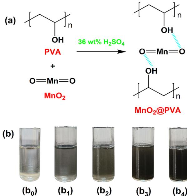
Fig. 1 (a) Interaction between MnO<sub>2</sub> and PVA. (b) Photo images of (b<sub>0</sub>) plane PVA, (b<sub>1</sub>) 1 wt% MnO<sub>2</sub>@PVA, (b<sub>2</sub>) 3 wt% MnO<sub>2</sub>@PVA, (b<sub>3</sub>) 5 wt% MnO<sub>2</sub>@PVA and (b<sub>4</sub>) 7 wt% MnO<sub>2</sub>@PVA gel electrolytes.
