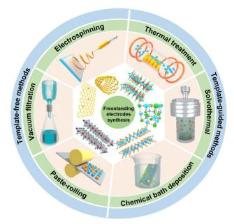
Fig. 2 Schematic diagrams of the active materials, template-free, and template-quided fabrication methods of the freestanding electrodes.
