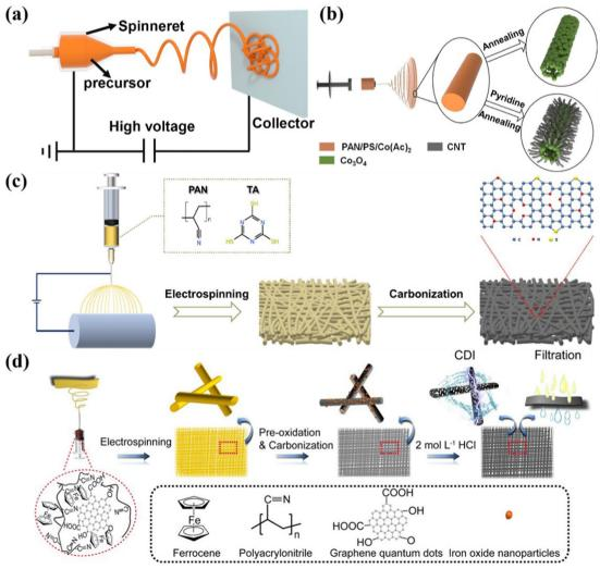
Fig. 3 (a) Schematic diagrams of the electrospinning process. Illustration of the preparation of the freestanding (b)  $Co_3O_4$ @CNF@CNT and (c) S/N codoped CNT electrodes, reproduced from ref. 88 and 89 with permission from Elsevier. (d) Schematic of the fabrication of graphene quantum dot modified CNT electrodes, reproduced from ref. 90 with permission from the American Chemical Society.
