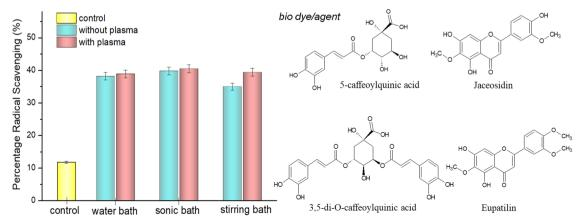
Fig. 5 SEM images and antioxidant capacity of dyed fabrics, and chemical structures of the bio-dye/agent from FAA extracts
