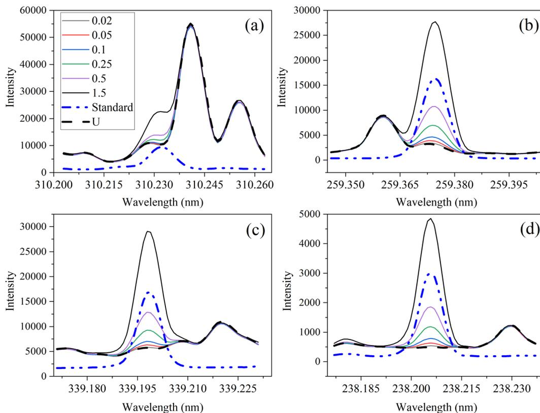
Fig. 1 Optical emission spectra of trace elements from 0.02 to 1.5  $\mu\text{g mL}^{-1}$  in 1000  $\mu\text{g}$  per mL U for (a) V 310.23 nm, (b) Mn 259.37 nm, (c) Zr 339.20 nm, and (d) Fe 238.20 nm compared to a standard ( $1 \mu\text{g mL}^{-1}$  multielement standard) and a 1000  $\mu\text{g}$  per mL U sample.
