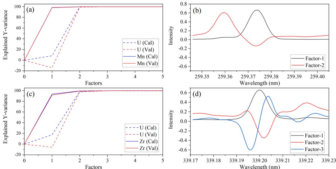
**Fig. 3** Explained variance and *X*-variable (nm) loadings plot for Mn 259.373 nm (a, b) and Zr 339.198 nm (c, d).
