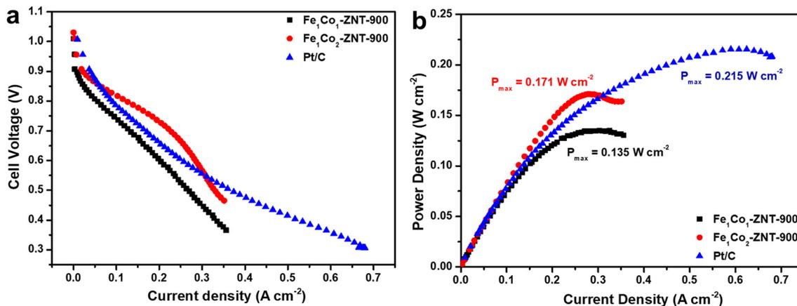
Fig. 7 (a) Polarisation and (b) power density curves obtained for  $\text{Fe}_1\text{Co}_1\text{-ZNT-900}$ ,  $\text{Fe}_1\text{Co}_2\text{-ZNT-900}$ , and Pt/C cathode catalysts in  $\text{H}_2/\text{O}_2$  AEMFCs [anode catalyst: PtRu/C. AEM: Aemion+® 15  $\mu\text{m}$ .  $T = 65^\circ\text{C}$ ].
