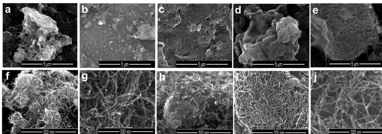
**Fig. 2** SEM images captured for (a and f) ZNT-900, (b and g) Fe-ZNT-900, (c and h) Co-ZNT-900, (d and i)  $\text{Fe}_1\text{Co}_1$ -ZNT-900 and (e and j)  $\text{Fe}_1\text{Co}_2$ -ZNT-900 catalysts at different resolutions.
