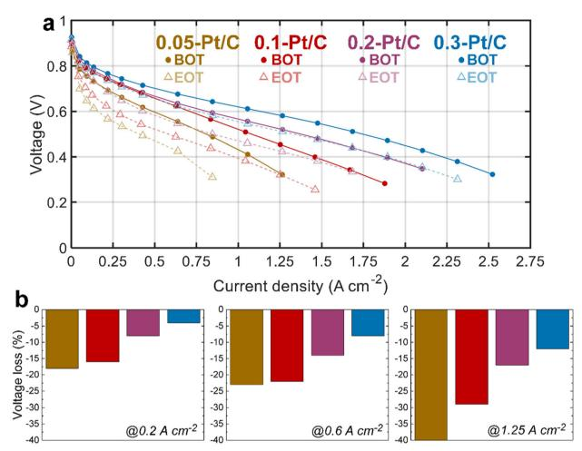
Fig. 1 (a) Polarization curves for the MEAs comprising 0.05-Pt/C, 0.1-Pt/C, 0.2-Pt/C and 0.3-Pt/C cathode CLs at BOT and EOT; (b) voltage losses of selected points at low (0.2 A cm<sup>-2</sup>), medium (0.6 A cm<sup>-2</sup>) and high (1.25 A cm<sup>-2</sup>) current densities.
