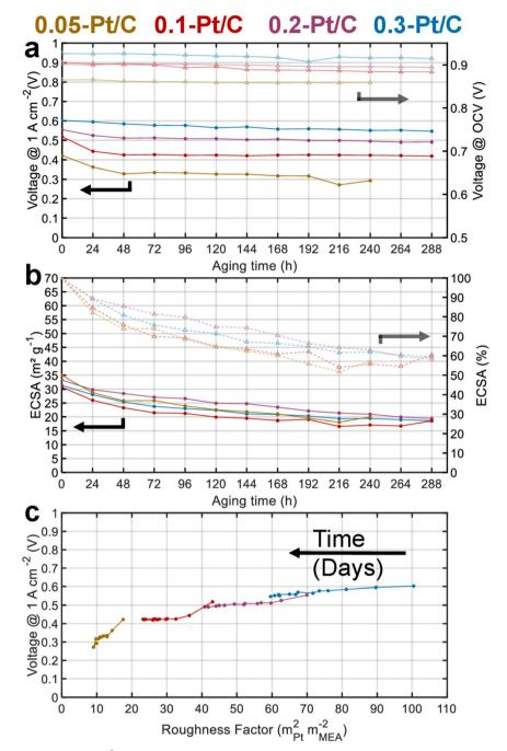
Fig. 2 (a) Cell voltages measured at 1 A cm<sup>-2</sup> during the daily characterization step and their OCV in the course of the AST; (b) ECSA mapping and its percentage loss; (c) cell voltage at 1 A cm<sup>-2</sup> vs. roughness factor, R.F., both values being measured in real-time along the 288 h of AST for 0.05-Pt/C, 0.1-Pt/C, 0.2-Pt/C and 0.3-Pt/C cathode CLs.
