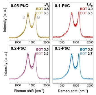
Fig. 8 Raman spectra for 0.05-Pt/C, 0.1-Pt/C, 0.2-Pt/C and 0.3-Pt/C cathode CLs at beginning of test (BOT) and end of test (EOT) coupled to their respective  $I_d/I_a$  ratio.
