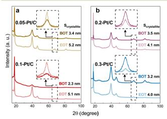
Fig. 7 Grazing incidence X-ray diffractrograms for the cathode CLs: (a) 0.05-Pt/C and 0.1-Pt/C and (b) 0.2-Pt/C and 0.3-Pt/C at beginning of test (BOT) and end of test (EOT) with their respective crystallite size values calculated at the highlighted graph region (Pt 220;  $2\theta \approx 68^{\circ}$ ).
